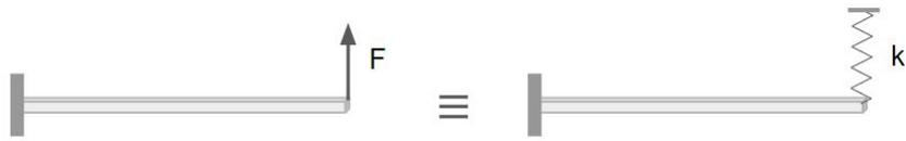
**Figure C-1:** Equivalent cantilever beam with a point force acting on its end  $F$
