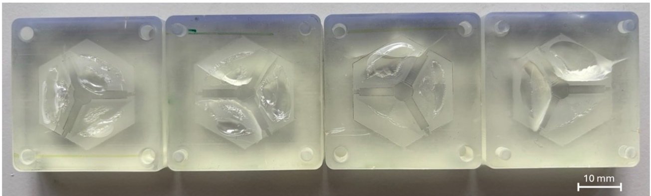
Fig. B.6. Samples of thermally fused moulds for the triple beam unit cells. Due to insufficient parallelism between the moulds, certain pressure/contact points started melting.
