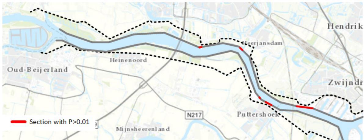
Figure E.10: Sections with with  $P(L > L_{max})_{section} > 0.01$  on the river Oude Maas.
