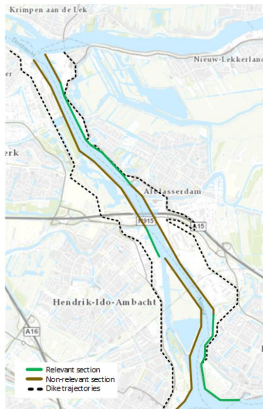
Figure E12: Relevant sections for flow slide on the river Noord.
