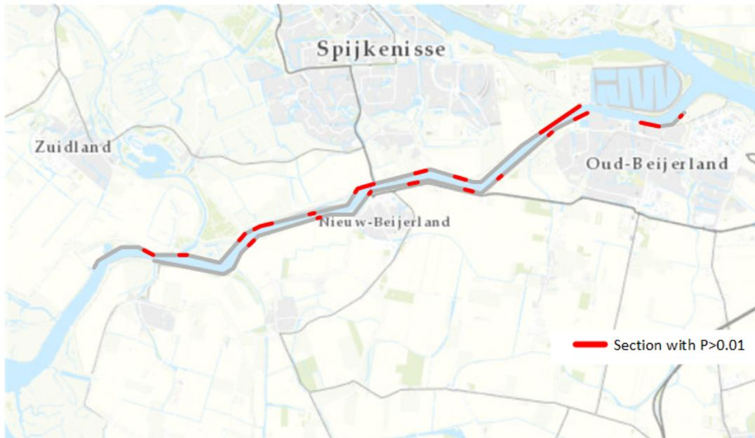
Figure E5: Sections with with  $P(L > L_{max})_{section} > 0.01$  on the river Spui.
