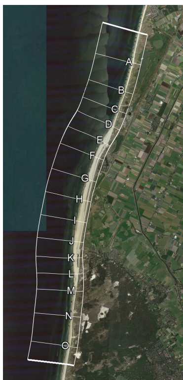
Figure 6.1: Google Earth image with the boundaries of the grid applied in the XBeach model and the location of the different transects. Modified from Google Earth.
