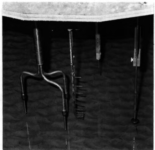
Photo 4, acoustical velocity and concentration probe (left) pump intakes (middle) electro magnetic velocity probe (right)
