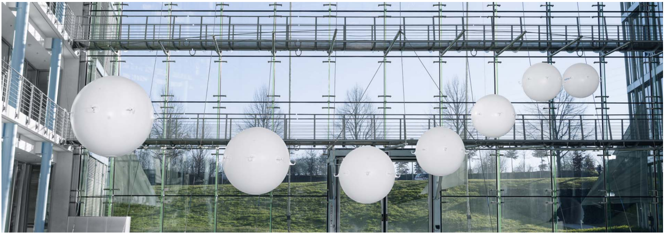
Figure 1: eMotionSpheres: an interactive infrared camera system enables both the formation and individual flight of the spheres.
