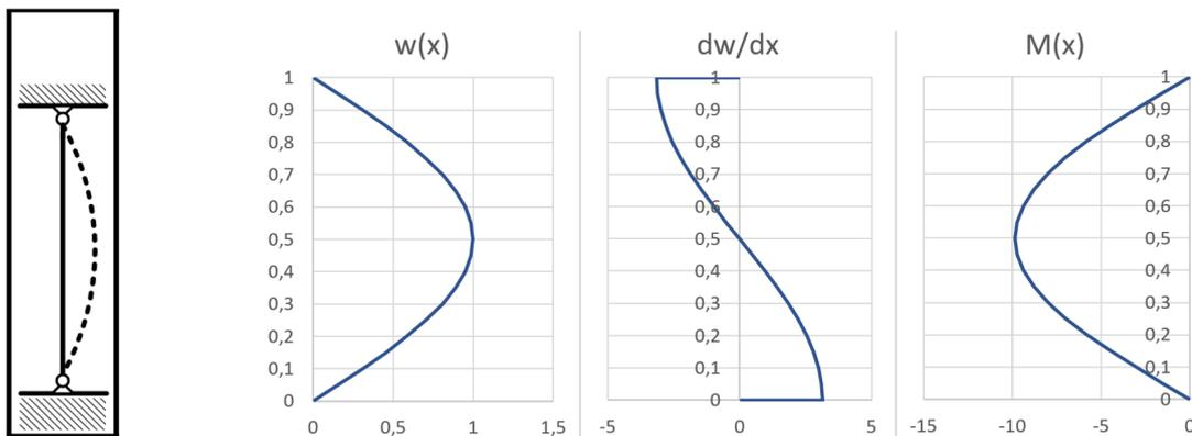
Figure 2.2: Displacement, curvature and moment lines for boundary condition set 1
