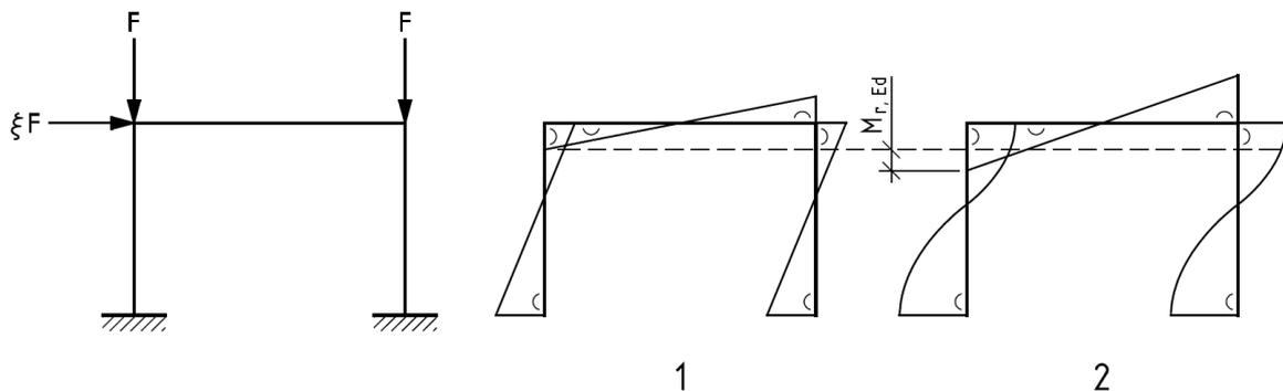
Figure 3.3: Sway frame: 1. first order elastic moment lines and 2. moment lines at failure
