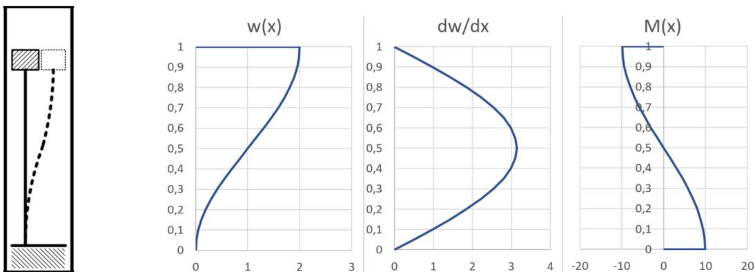
Figure 2.5: Displacement, curvature and moment lines for boundary condition set 4
