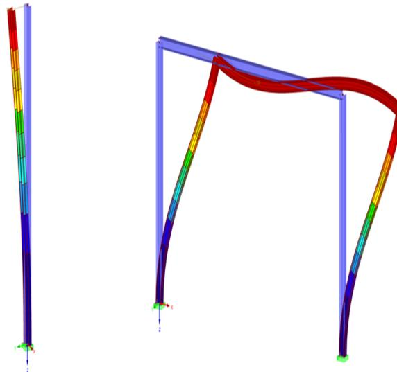
Figure 1.1: Single column buckling (left) and frame buckling (right)
