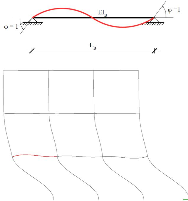
Figure 4.7: Beam in sway frame
