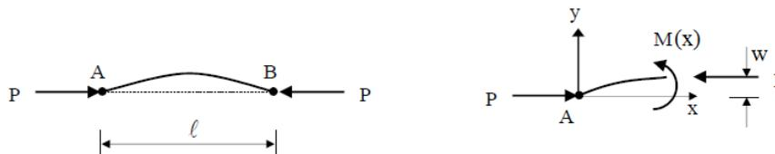
Figure 2.1: Single pinned pinned column and small segment
