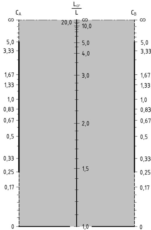
Figure 3.5: Elastic effective buckling length or elastic fixed columns in sway frames
