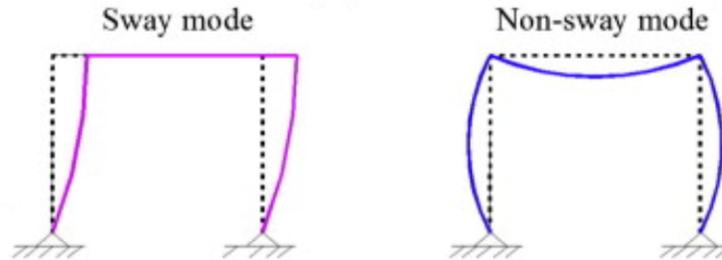
Figure 1.2: Sway mode (left) and non sway mode (right)
