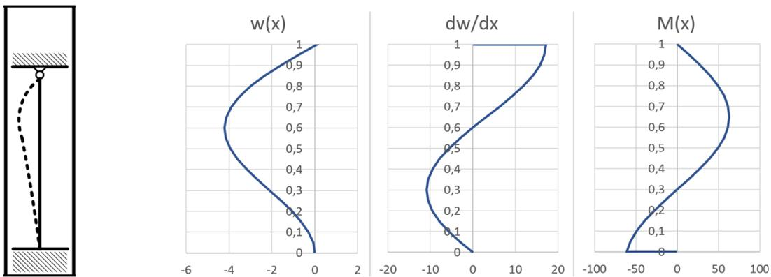
Figure 2.4: Displacement, curvature and moment lines for boundary condition set 3
