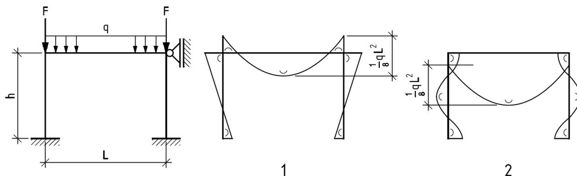
Figure 3.7: Non Sway frame: 1. first order elastic moment lines and 2. moment lines when the structure buckles
