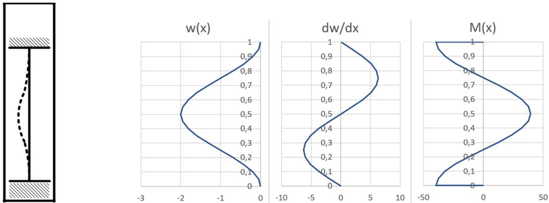
Figure 2.3: Displacement, curvature and moment lines for boundary condition set 2
