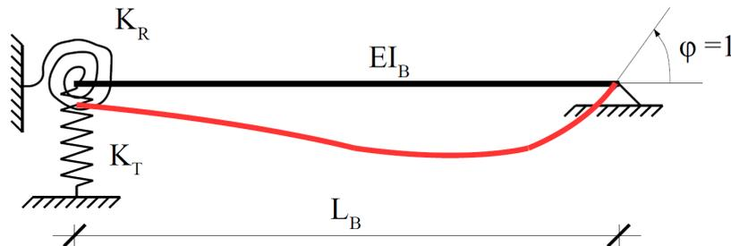
Figure 4.5: The effective rotational parameter case with general support condition at far end
