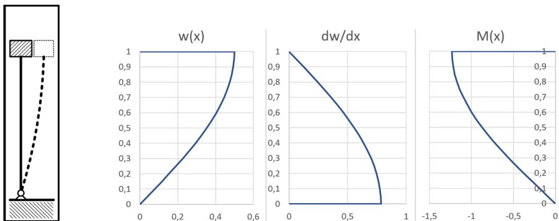
Figure 2.7: Displacement, curvature and moment lines for boundary condition set 6
