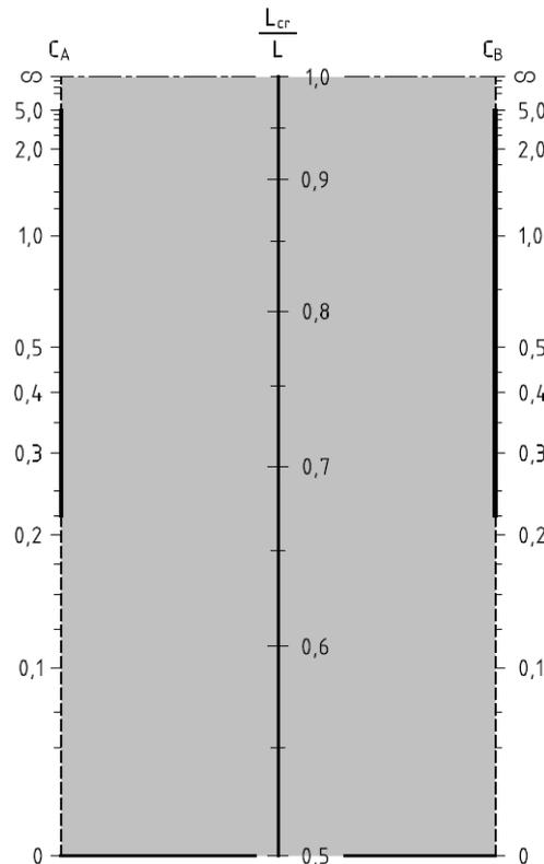
Figure 3.9: Elastic effective buckling length or elastic fixed columns in non sway frames
