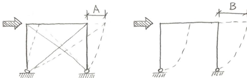
Figure 1.3: Braced frame and unbraced frame for checking of the corresponding frame is a sway frame
