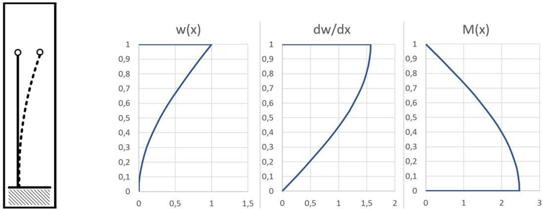
Figure 2.6: Displacement, curvature and moment lines for boundary condition set 5
