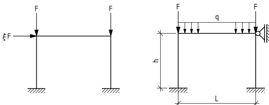
Figure 1.4: Situation 1 or Sway frame (left) and situation 2 or non sway frame (right)
