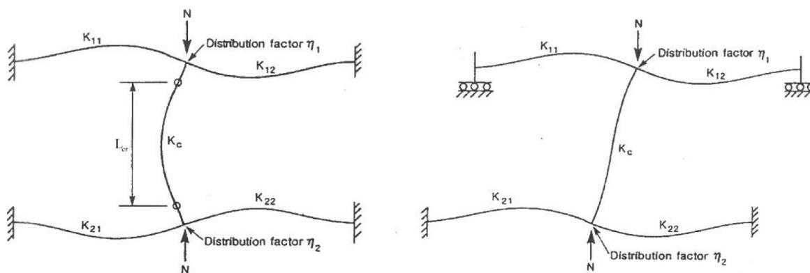
Figure 4.4: Theoretical model for non-sway and sway mode
