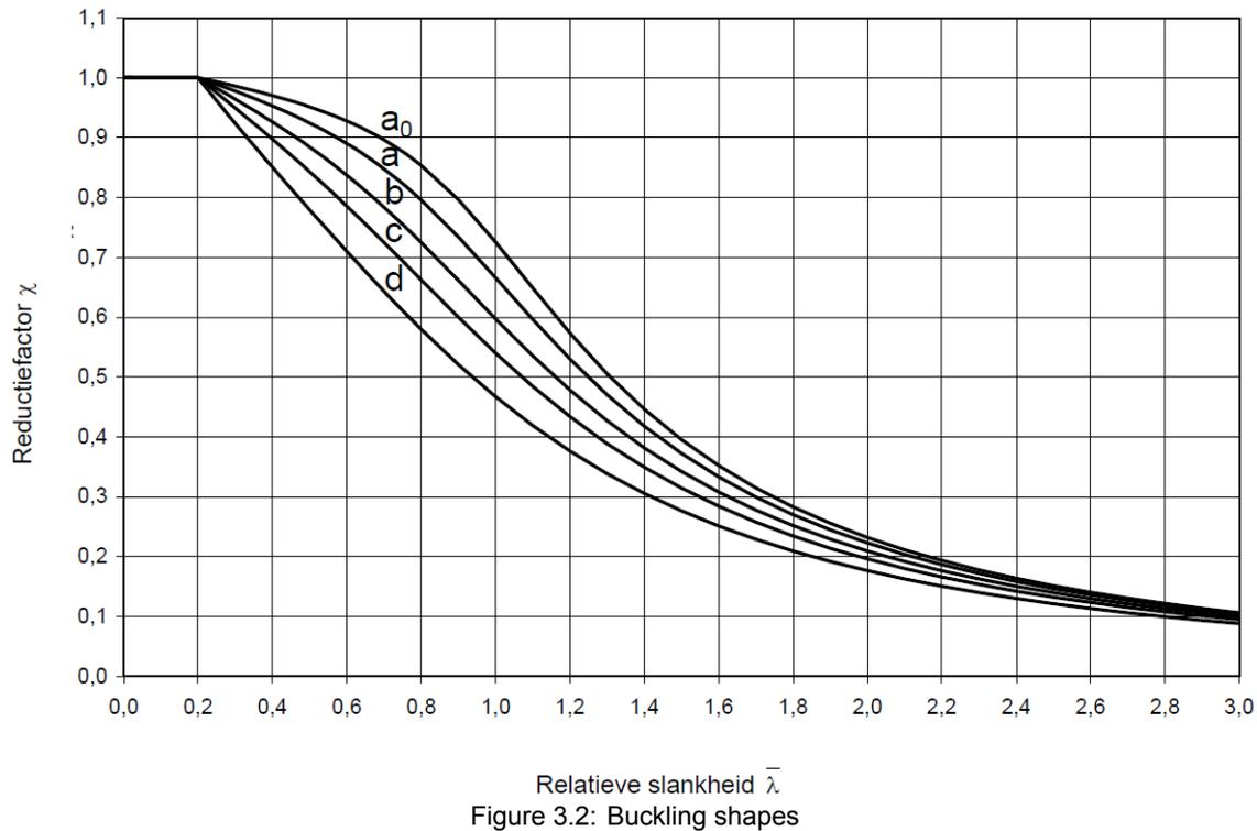
If the buckling shape is known the imperfection factor  $\alpha$  can be determined from the table below
