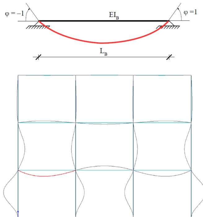
Figure 4.6: Beam in non- sway frame
