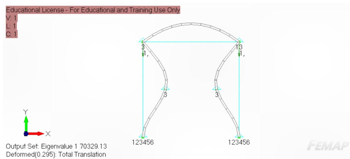
Figure 4.2: Linear buckling analysis result for situation 2
