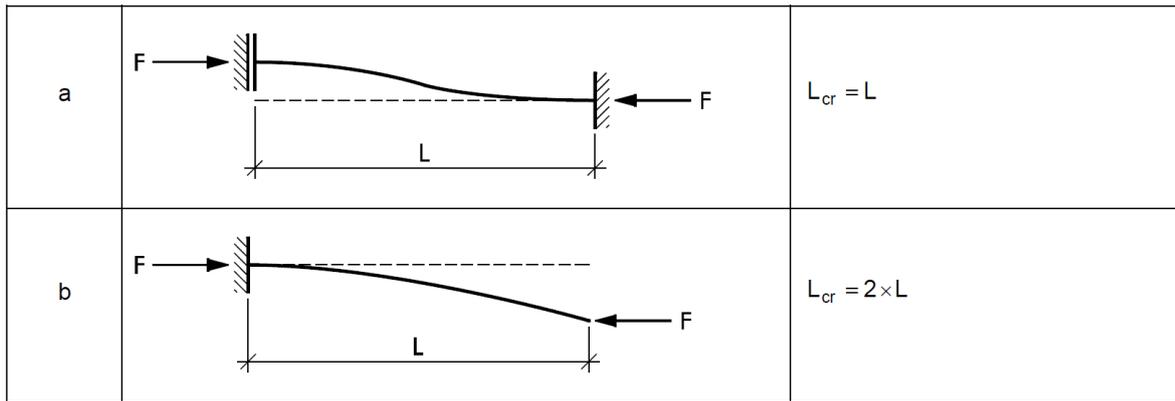
Figure 3.4: Effective buckling lengths with fixed columns in a sway frame
