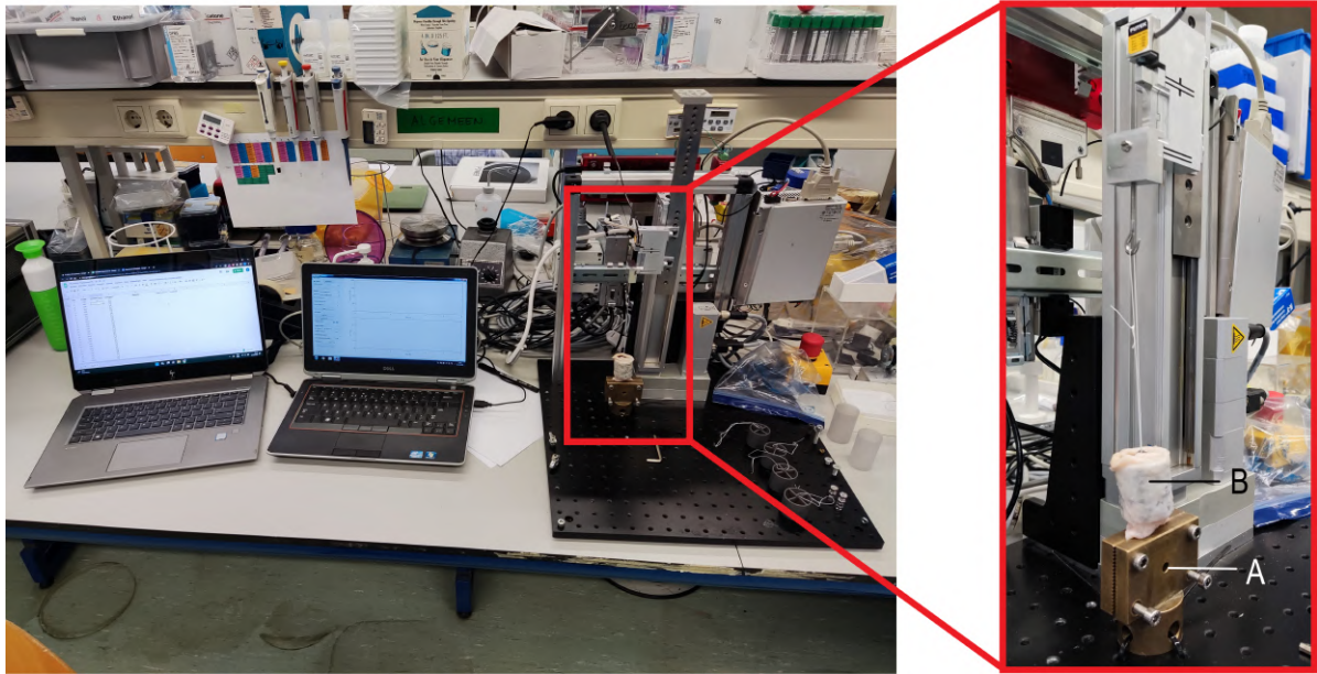
Figure 3.12: Setup of Experiment 3, with on the right side A) clamp and B) colon with one test stent inside.
