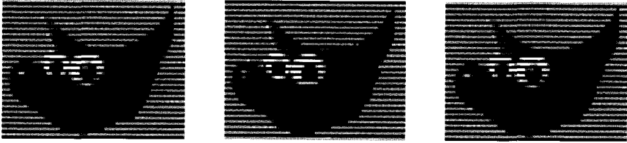
Figure 5.1: Three successive fields of an interlaced video sequence.
