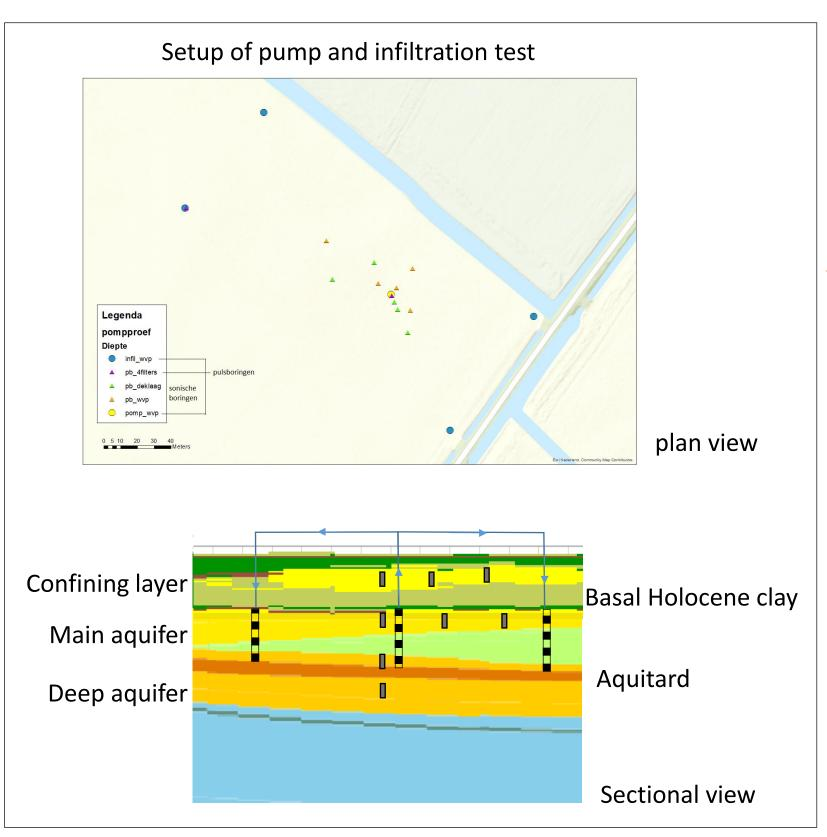
Exploratory model simulations have shown that 1) a reliable estimate of the resistance requires the measurement of a drawdown above the clay layer, and 2) only a small drawdown will develop above the clay layer even though the pumping will run for several months. This means that a small drawdown due to the pumping has to be separated from the background influences.
