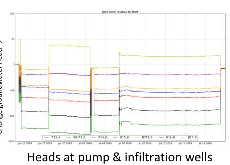
during tests with varying infiltration
