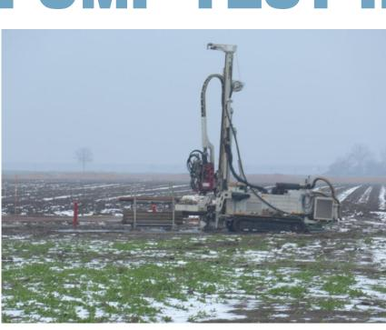
The pump test setup consisted of one pumping well and four infiltration wells, two multi-level piezometers, five piezometers screened in the pumped aquifer, and five screened in the sandy part of the confining layer. The water pumped was injected using different combinations of the infiltration wells. This setup and the variation in flow will allow to assess the spatial variability at the scale of the test site.
