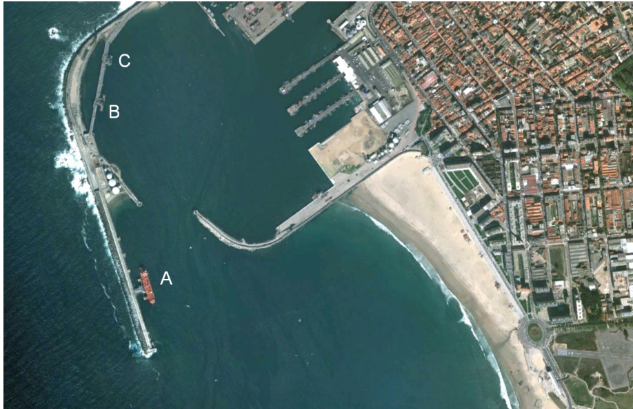
Figure 4.1: Satellite picture of the Port of Leixões area, showing the oil terminal and its three berths (© GeoEye; DigitalGlobe)
