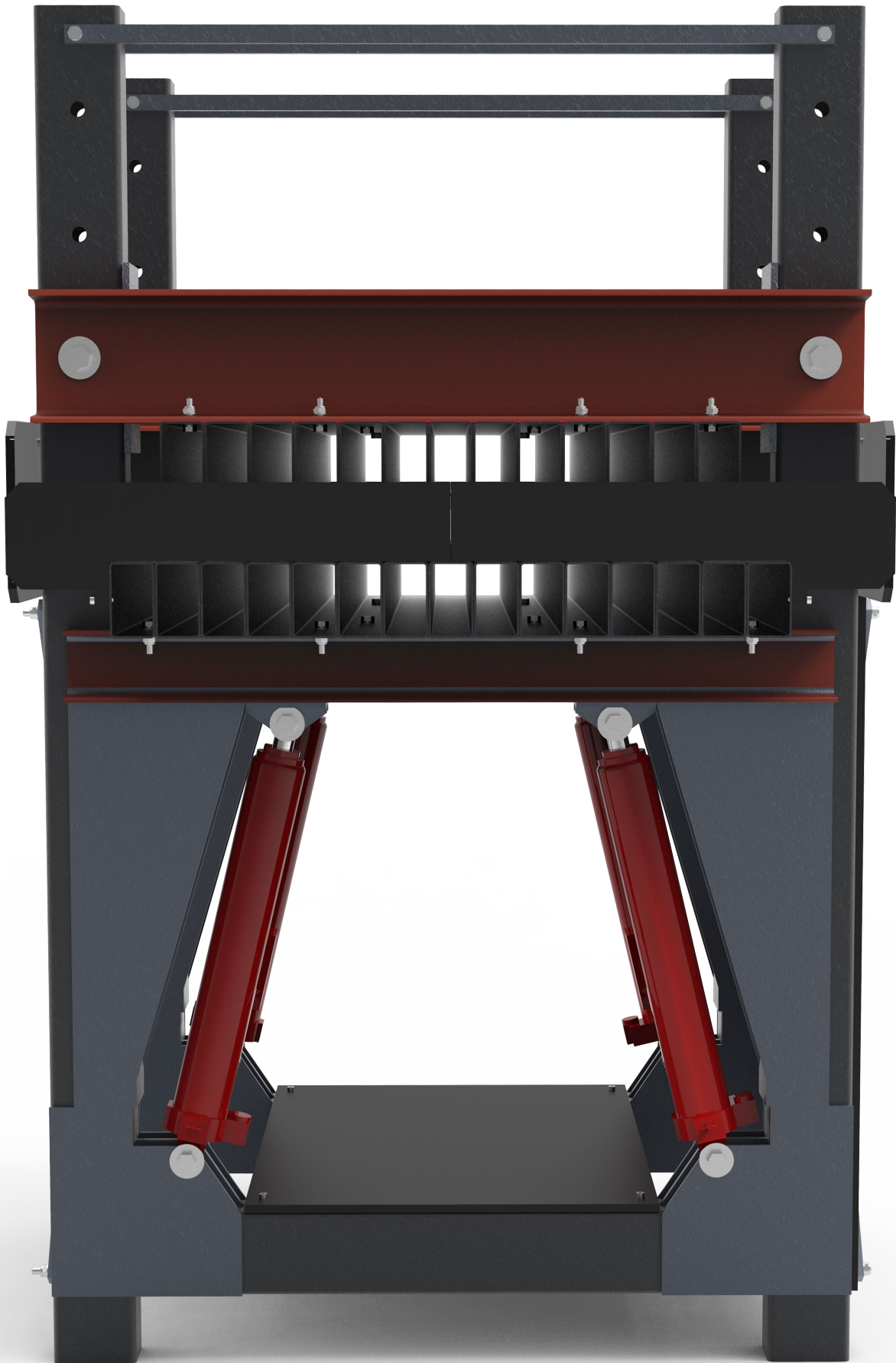
Figure 8-1, Improved Plastic plate Press Design Render- Figure by Mark Bachrach
