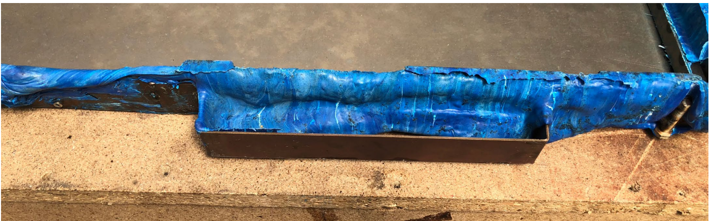
Figure 7-4, Plastic stuck in mould handle - Picture by Mark Bachrach
