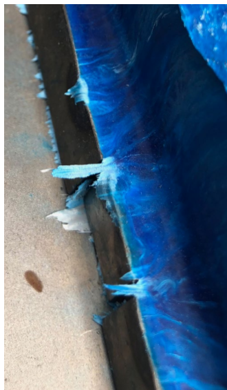
Figure 7-6, Cut-off-edge bending upwards - Picture by Mark Bachrach
