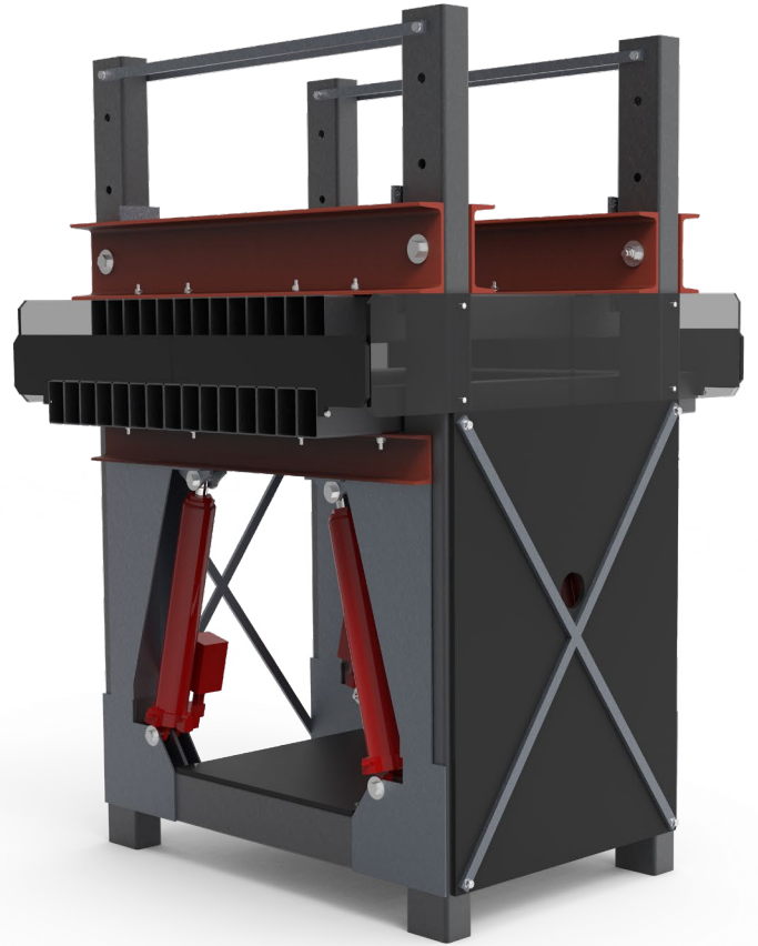
Figure 8-2, Improved Design - Closed 'Press Guards' - Figure by Mark Bachrach
