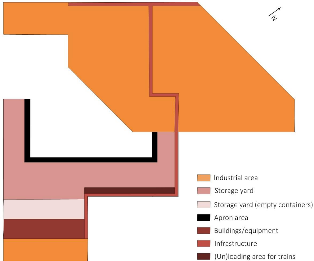
FIGURE L-3: THE LAYOUT OF THE TRANSSHIPMENT PART OF THE PORT (FIGURE IS ROTATED)
