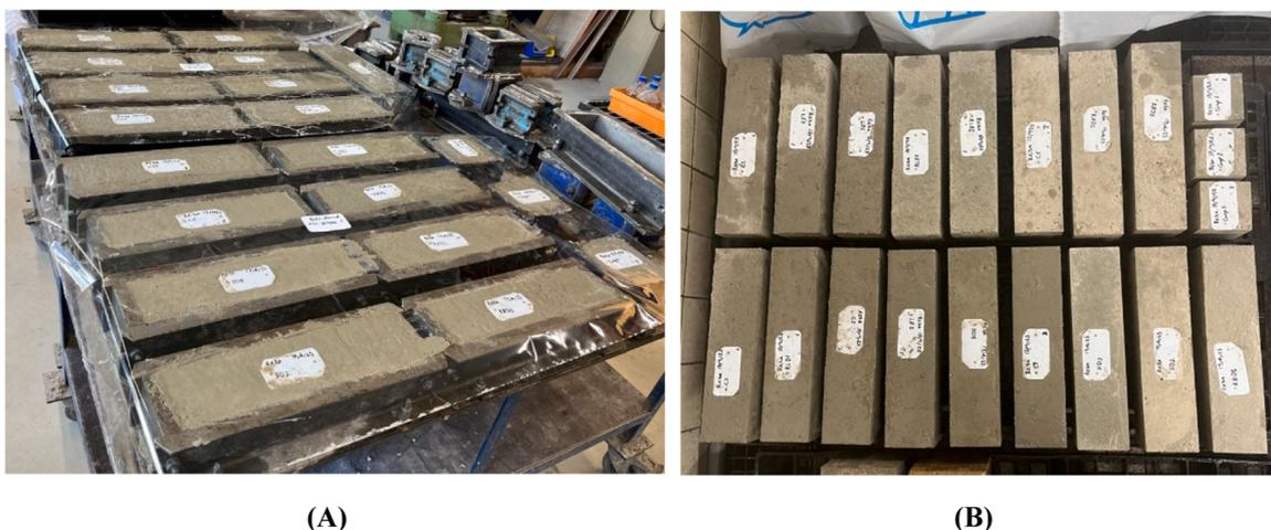
**Fig. 2.** Curing of the concrete prisms: (a) under plastic sheets, before unmoulding; and (b) in the moisture chamber, after unmoulding.
