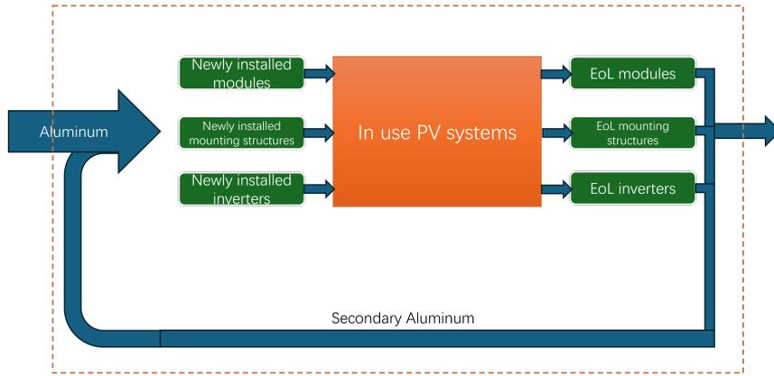
Figure 2.1: Diagram of the flow of aluminum in PV system
