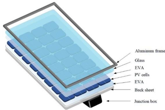
Figure 1.1: PV module structure [14]
