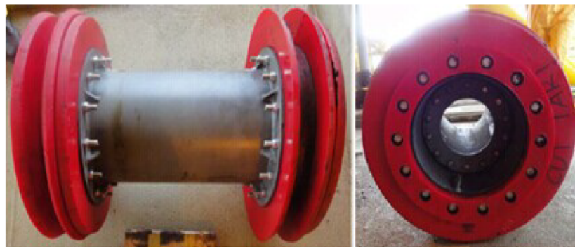
Figure 1.2: Picture of a conventional by-pass pig, reproduced from [3]
