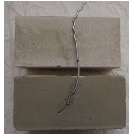
Tie in CS masonry couplets
