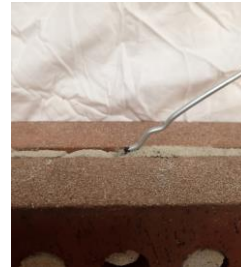
Tie in clay masonry couplets
