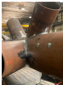
Figure 3.7: Example of a circular hollow section connection
