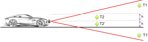
Fig. 4: Figure depicting the problem with ambiguous target heights, the red lines indicate the beamwidth in elevation, h is the height of the radar from the road, and T1/T2 are the detected targets.
