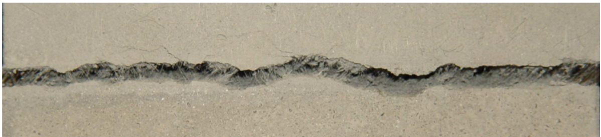
(a) Interfacial tensile test of a sandblasted specimen showing bridging fibres [28].
