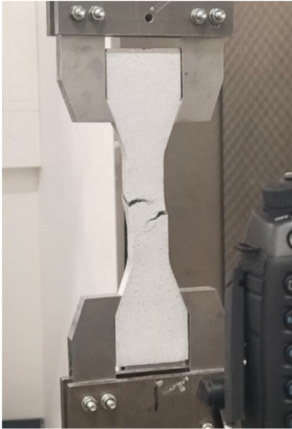
(a) Dogbone specimens tensile test setup [21].
