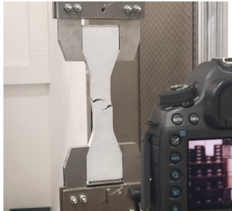
(a) Dogbone tensile test setup after testing from [21].
