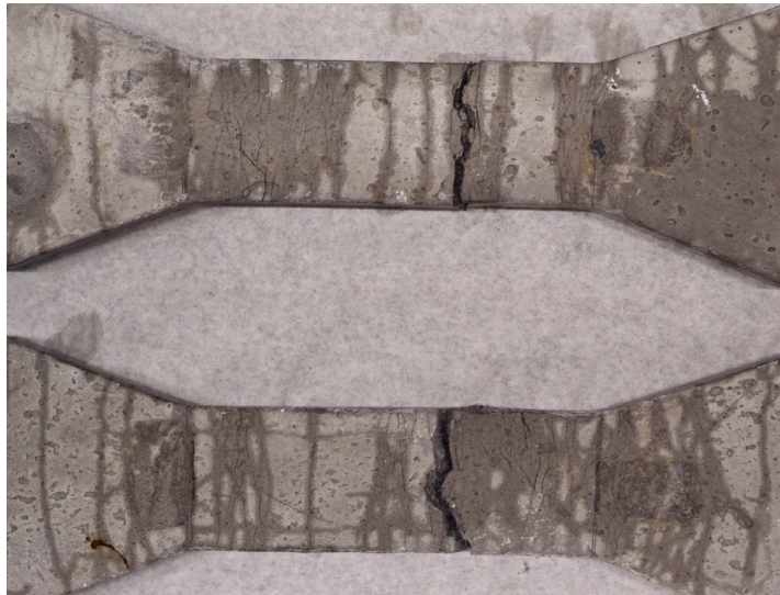
Figure 4.7: SHCC dogbone specimens after the tensile test [21].
