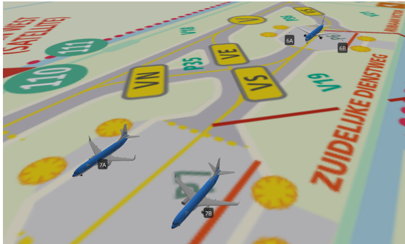
Figure 3.12: Each station can accommodate two narrowbodies, or one widebody aircraft
