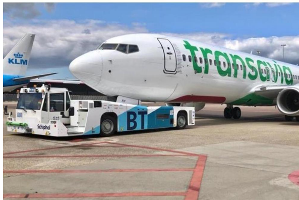
Figure 1.4: A TaxiBot connected to a Transavia Boeing 737 at Schiphol (Ground Handling International, 2022)
