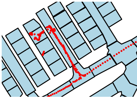
Figure 3.3: GPS drift at a stand causing radar labelling issues
