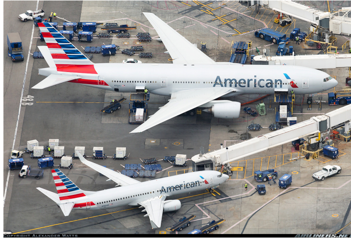
Figure 1.2: A Boeing 737 (narrowbody, bottom) and Boeing 777 (widebody, top) next to each other (Watts, A (Airlines.net), 2013)
