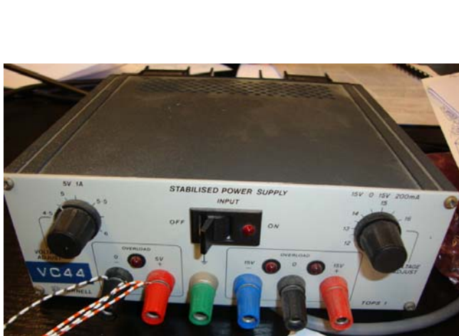
Figuur B5.8: Farnell Stabilised Power Supply
