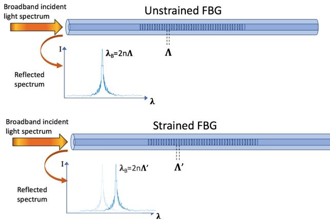
Figure 1.4: The principle of operation of uniform FBG sensors under uniform strain fields.  $I$  is the intensity of the reflected light,  $\lambda$  is the wavelength domain,  $\lambda_B$  is the peak wavelength of the reflected light,  $n$  is the effective refractive index of the core, and  $\Lambda$  and  $\Lambda'$  are the grating periods of the unstrained and strained FBG respectively.
