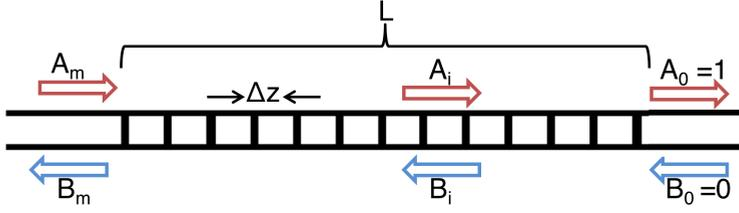
Figure 3.1: Schematic view of the FBG structure.
