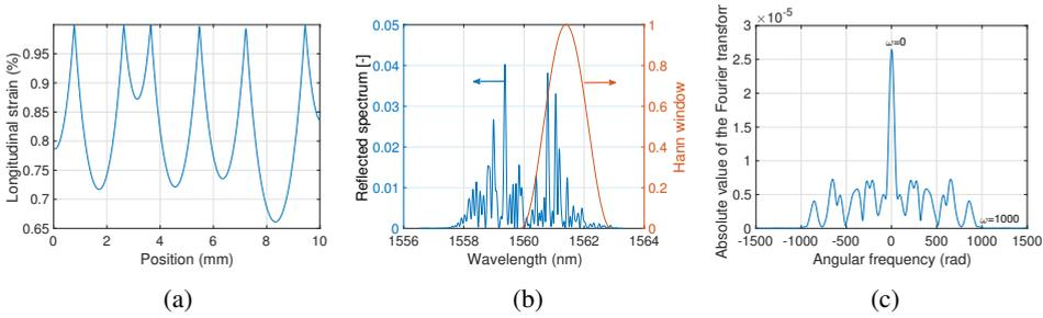
Figure 7.4: (a): Strain distribution along the length of the sensor when subjected to 6 transverse cracks, at  $\sigma = 250\text{MPa}$  (b): Reflection spectrum of a sensor near six cracks and the scaled Hann window. (c): Fourier transform of the windowed side-lobes of the reflection spectrum.
