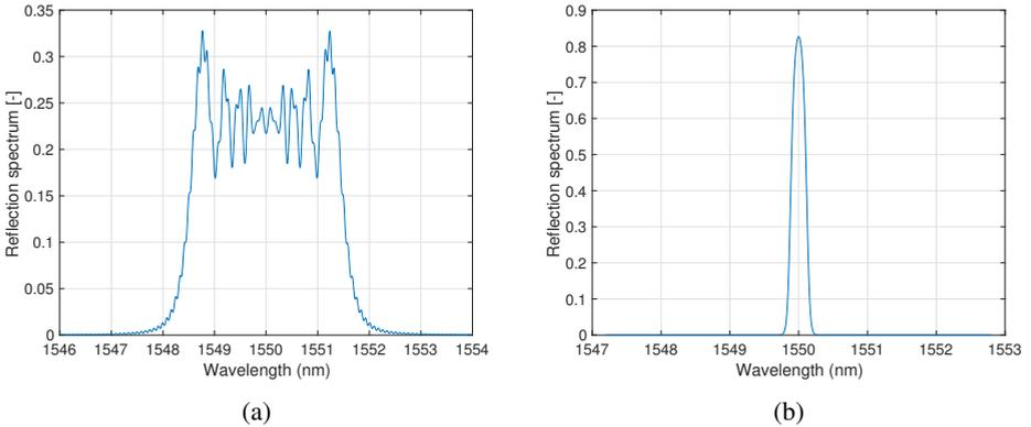
Figure 2.2: (a): The calculated reflection spectrum from a chirped Bragg grating with a chirp rate of  $d\lambda_B/dz = 3.34$  nm/cm. (b): The calculated reflection spectrum of a Gaussian apodized FBG sensor with fully suppressed side-lobes.
