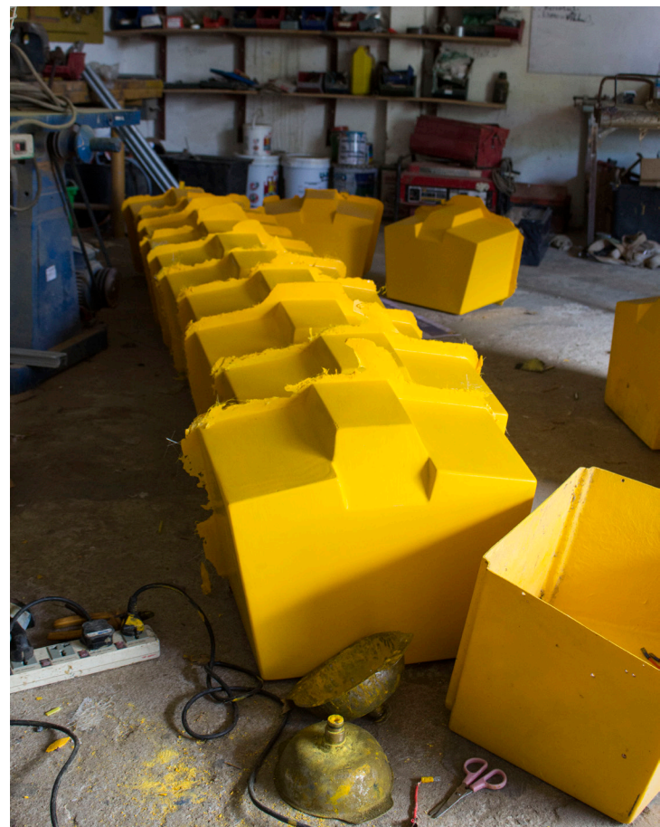
figure 29. The front of the large battery box before finishing.
