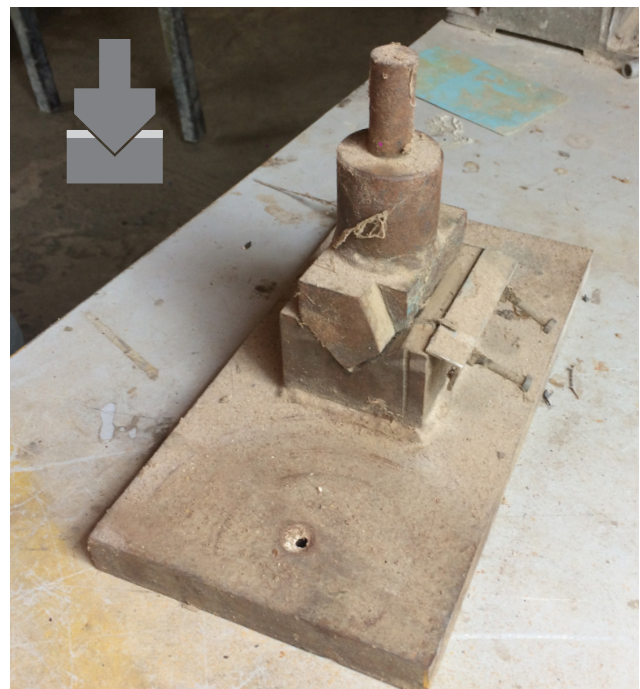
figure 55. Punch and die that can be recovered
