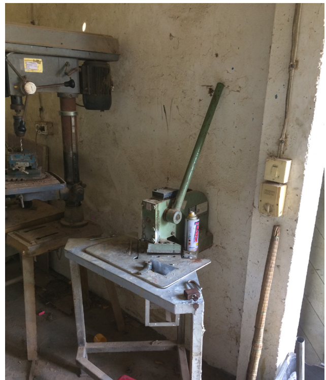
figure 62. Kamworks' manual corner notcher
