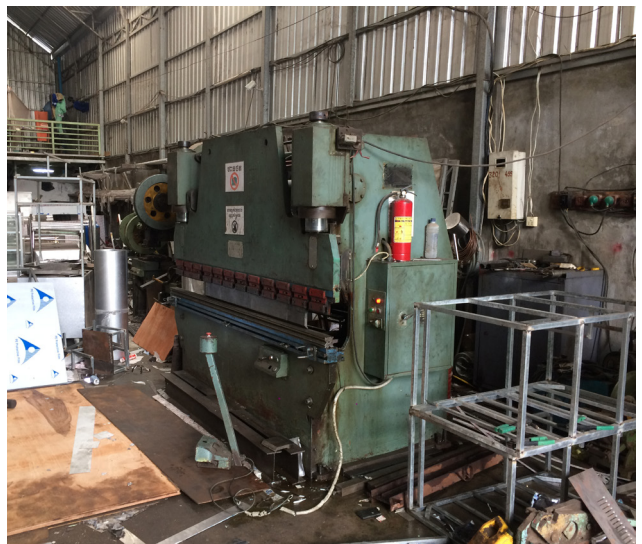
figure 72. The hydraulic press brake in the Phnom Penh factory
