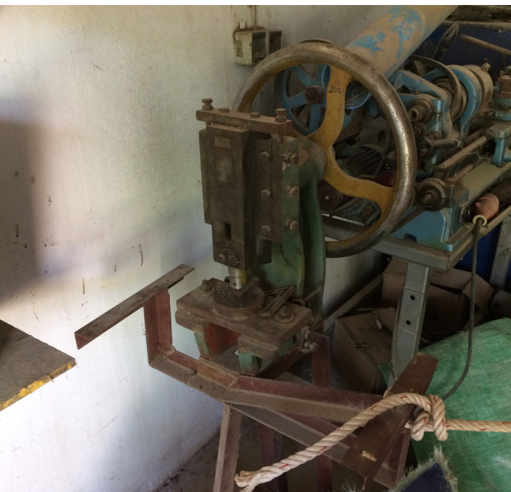
figure 54. The manual sheet metal punch in Kamworks' workshop
