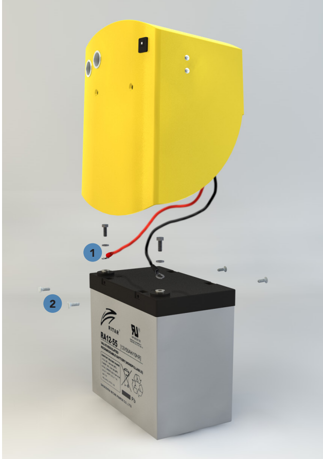
figure 50. Exploded view regular battery box
