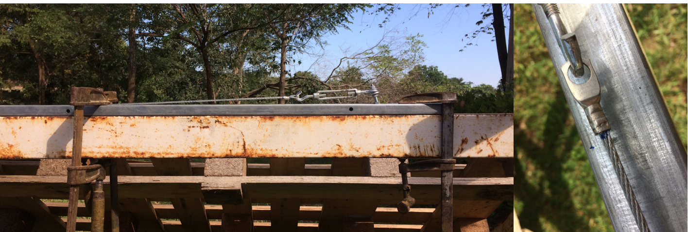
figure 97. Durability test cable lug
