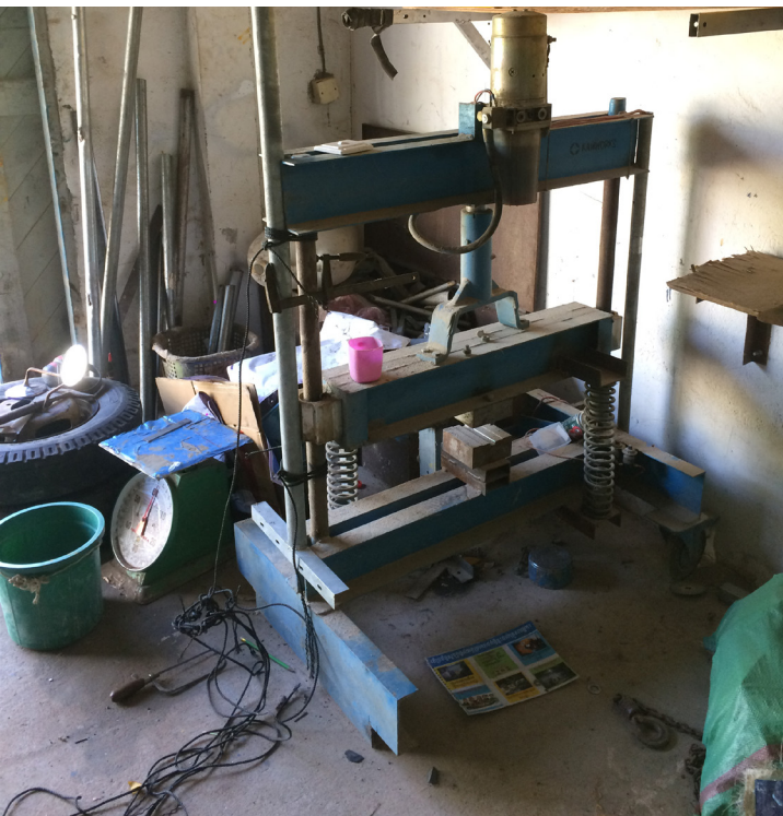
figure 61. Kamworks' hydraulic press
