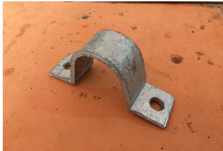
figure 68. Uncarefully finished parts
