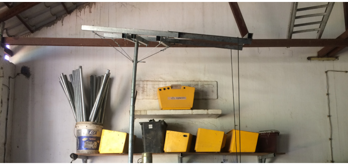
figure 89. Applying a load of 20kg at the end of the expansion
