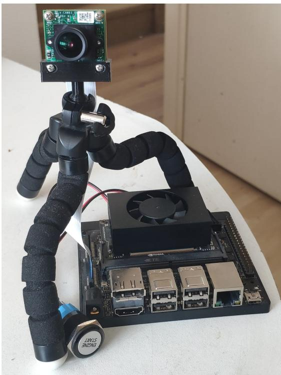
Figure 6.1: Nvidia Jetson Xavier NX with MIPI-CSI camera.
