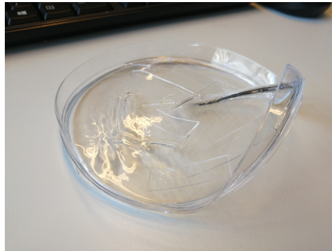
Figure 3.6: A twisted petri dish. The petri dish became soft in the oven for 1h at 90 degrees Celsius. Yet it was not sticky or melted
