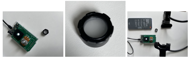
Figure 3: All components of the experiment, Redmi Note 10 as receiver, Tri-LED with Arduino and Diffuser as transmitter and a Tripod to hold the smartphone still
