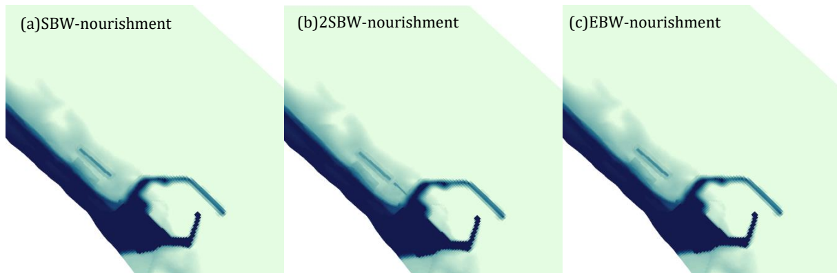
Figure 4.32: Schematisation of the interventions considered. (a) Submerged breakwater-nourishment: the submerged breakwater has dimensions 250m x15m and crest level at -0.5m MSL. (b) Set of submerged breakwaters-nourishment: the submerged breakwaters have dimensions 250m x15m and 110m x 12m, the crest level is at -0.5m MSL and the gap spans for 30m. (c) Emerged breakwater-nourishment: the emerged breakwater has dimensions 250m x15m and crest level at MSL. In all the figures the submerged nourishment (11000m 3 ) was simulated with the same characteristics.
