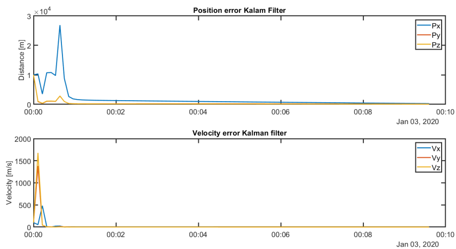
Figure E31: First observation arc for satellite 10793U, where the position and velocity difference between the SGP4-based reference state and EKF solution per epoch is visualised, for each separate element. Starting with an initialise covariance matrix.
