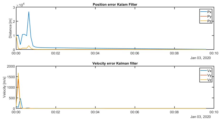
Figure F.19: First observation arc for satellite 10793U, where the position and velocity difference between the SGP4-based reference state and EKF solution per epoch is visualised, for each separate element.
