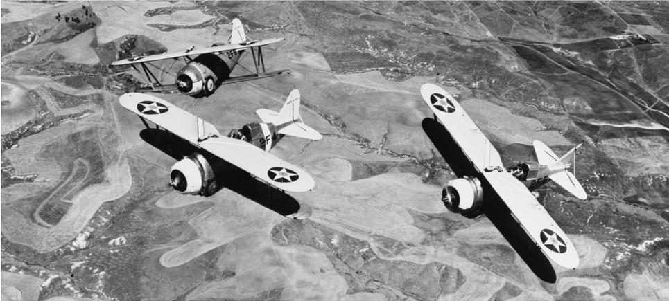
**Figure 6.1** Three Northrop Grumman F2F-1 fighters in steady, aerobatic, formation flight, 1939<sup>1</sup>. The leader is trimmed in straight and level flight, while the followers are trimmed in steady, asymmetric flight with forward slip.
