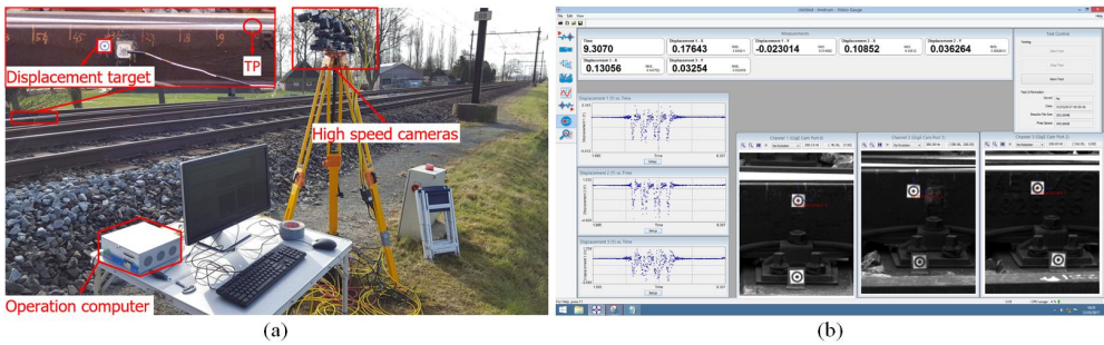
Figure 2.4. Wayside monitoring. (a): System setup; (b): The screen of displacement measurements.
