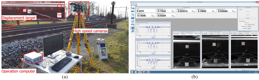
Figure 2.6. Wayside monitoring. (a): system setup; (b) Screen of displacements measurement.
