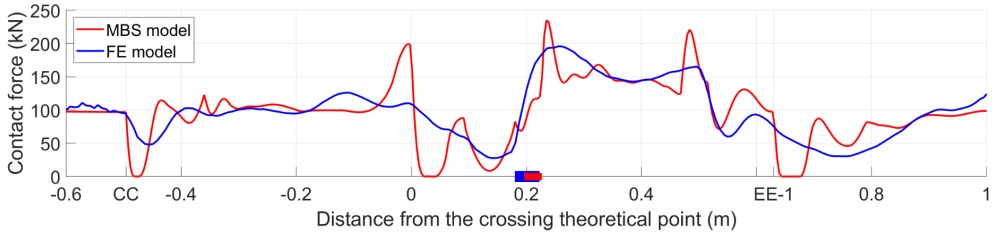
Figure 3.9. Comparison of the vertical wheel-rail contact forces.
