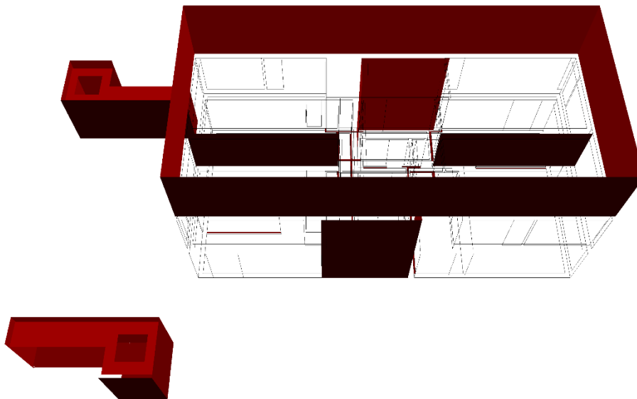
Fig. 9. Wrong space boundary connection geometries in red for the duplex model. Some boundaries are misplaced. Some boundaries do not have the appropriate geometry. Strangely, some space boundary geometry consists of wall footprints.
