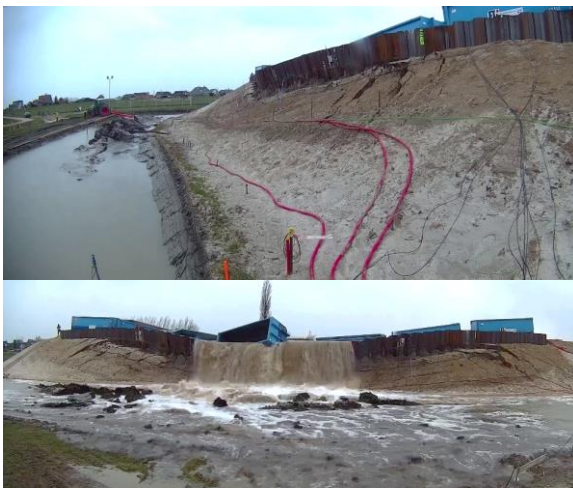
Figure 12 Photo's of sheet pile dike during failure, just before (a) and during (b) flooding.
