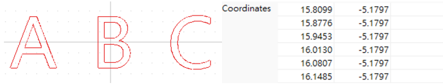
Figure 4.5: Vector type 2-dimensional pattern visualization and the coordinates of this pattern for controlling the galvanometers in BeamConstruct software.
