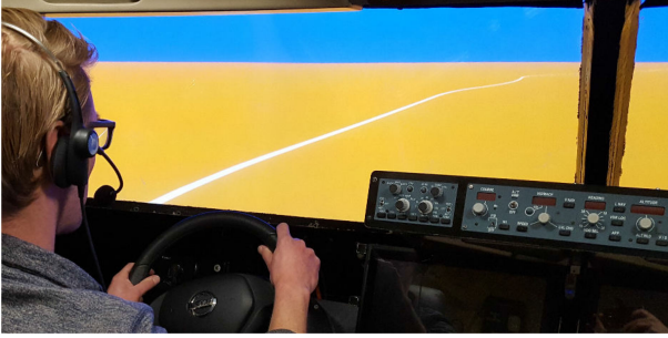
Fig. 3. Picture of the experimental setup during the experiment, inside the SIMONA research simulator (SRS) of TU Delft. This simulator is often used for aviation research, but was adapted to driving for the current experiment.
