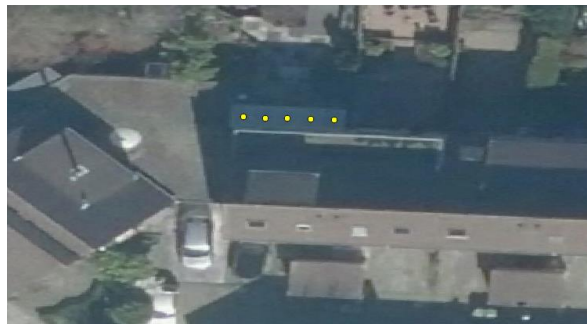
FIGURE 31: PV PANEL WHICH LIES IN SHADOW
