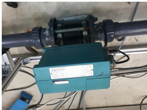
Figure A.31: Flow meter attached to the inflow
