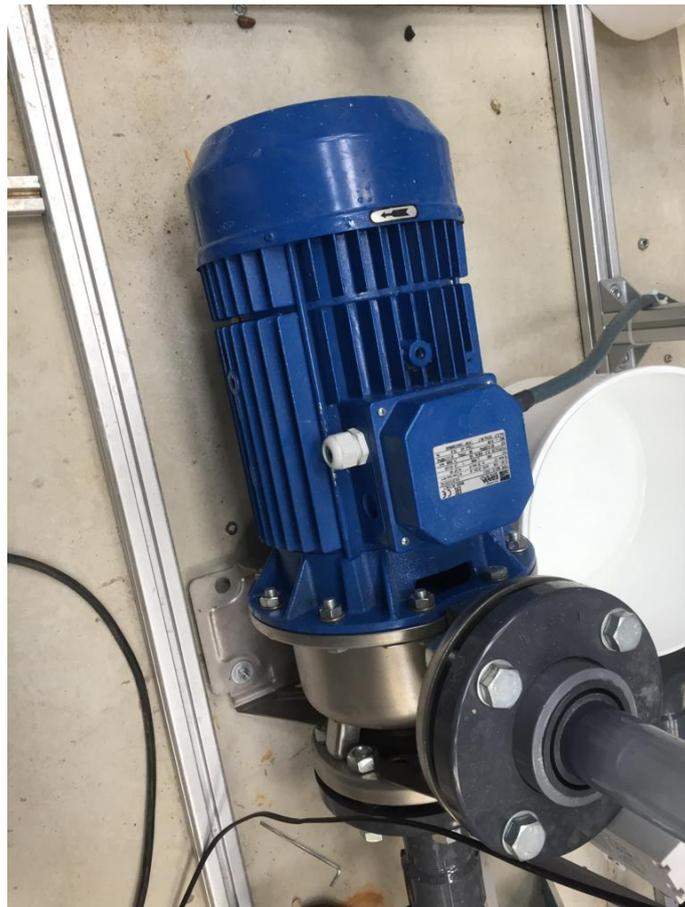
Figure A.5: Centrifugal pump
