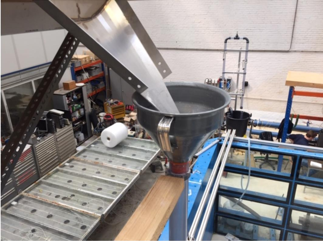
Figure A.9: Hopper used for guiding particles into stream
