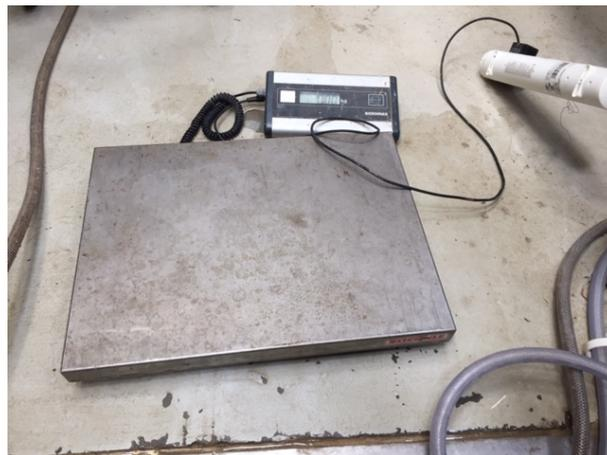
Figure B.4: Scale used density tests
