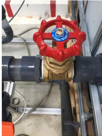
Figure A.29: Valves used for altering split ratio of the cyclone.
