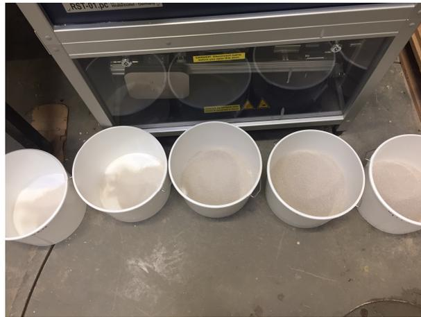
Figure B.3: Sand used for density tests
