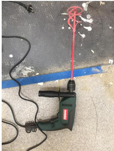
Figure A.33: Drill used for mixing suspension
