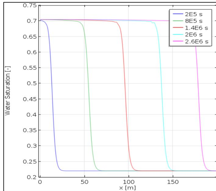
Figure 21 - Water Saturation Profile before DME Injection
