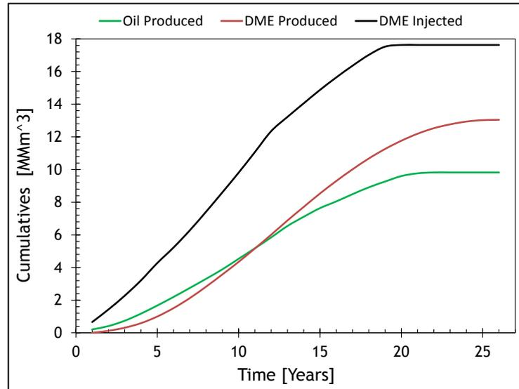
Figure 37 - Cumulative Oil Production, DME Production and DME Injection (Incremental due to DME Injection)
