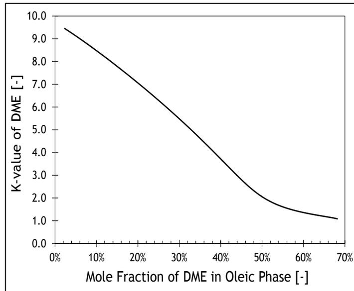
Figure 22 – K-value (mol-fraction DME in oleic divided by DME in Aqueous Phase, i.e. DME Partitioning Coefficient between the Aqueous and Oleic Phase)
