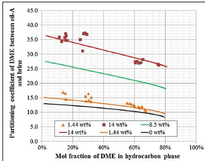
Figure 14 - DME Partitioning between Oil and Brine (of varying salinity) at Reservoir Conditions: 343 K and 17,236 kPa: Marker Points Corresponds to Experiments and Solid Line Corresponds to CPA Model (Ratnakar et al., 2016b)
