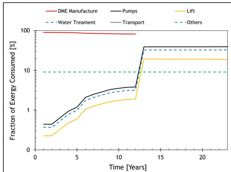
Figure 41 - Fractions of the Consumed Exergy in different Components of the Considered System (Rate)
