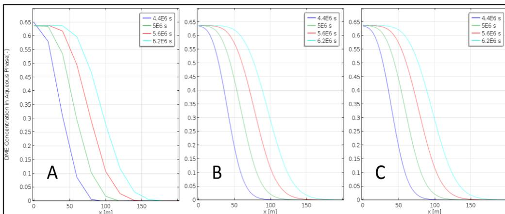
Figure 29 – DME Concentration in the Aqueous Phase for Mesh Size 10 m (A), 1 m (B) and 0.1 m (C)
