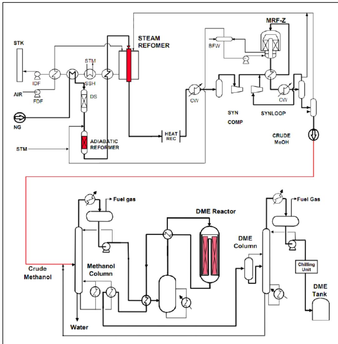
Appendix C - Concept of Slurry Phase DME Reactor (Inokoshi *et al.*, 2005)
