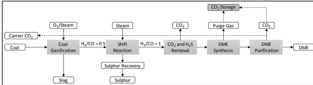
Figure 8 - Direct DME Synthesis Process from Coal (Japan DME Forum, 2011)
