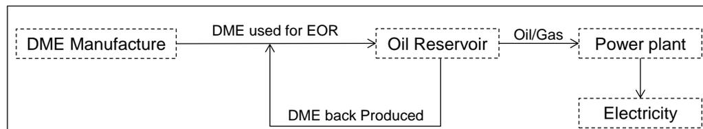
Figure 36 - Current Conventional Method of using DME for Enhanced Water Flood
