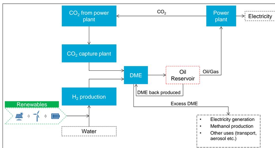
Figure 44 - Innovative Ways of Producing DME and its Integration into the Oil Production System
