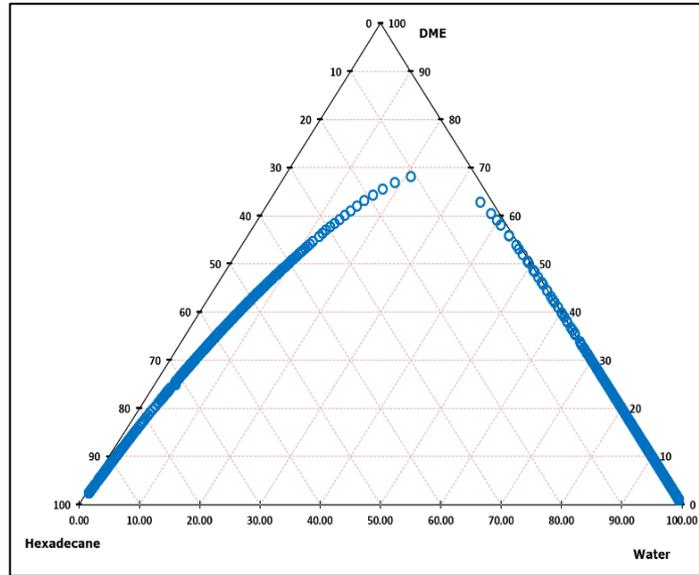
Figure 18 - Ternary Diagram for DME/Hexadecane/Water System
