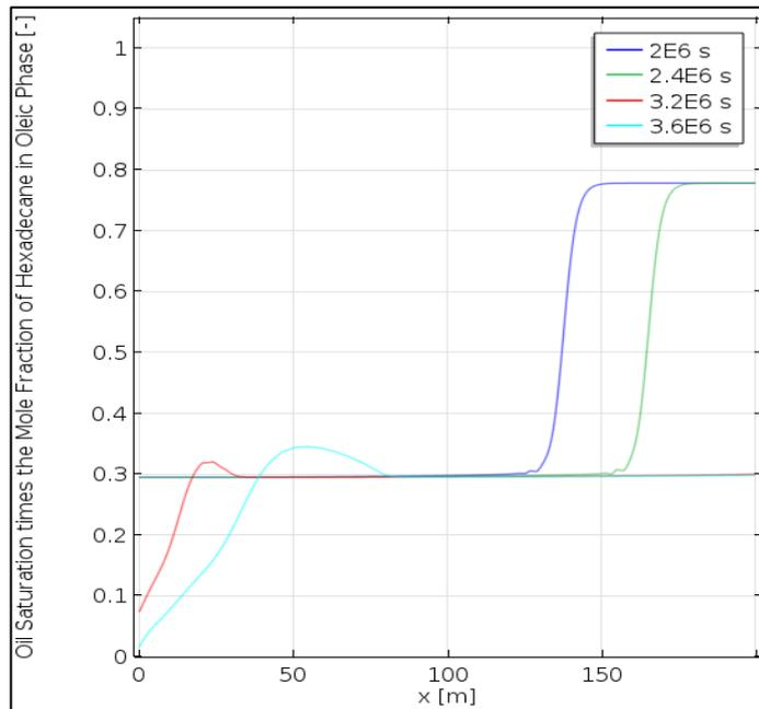
Figure 26 - Oil Saturation times the Mole Fraction of Hexadecane in the Oleic Phase
