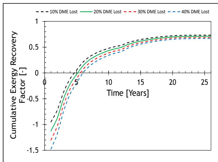
Figure 43 - The Cumulative Exergy Recovery Factor as a function of Time (Sensitivity to DME Lost)
