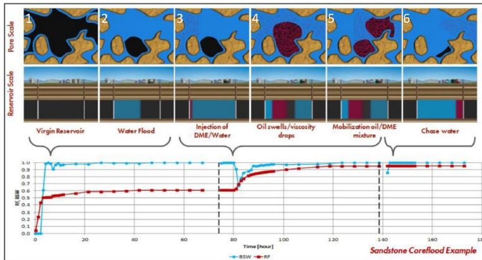
Figure 11 - Simplified Visualization of the DME Process with Phases of Activities Mapped Against the Experimental Results of Sandstone Core flood Undergoing the same Sequence of Flooding Events (Parsons *et al.*, 2016)
