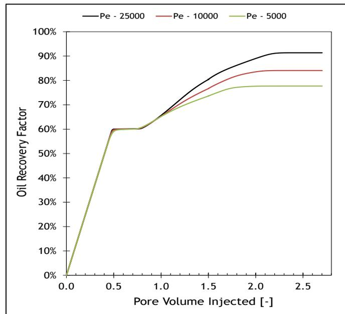
Figure 31 - Oil Recovery Factor for Different Peclet Numbers [A -  $N_{pe} = 5000$ ; B -  $N_{pe} = 10000$ ; C -  $N_{pe} = 25000$ ]
