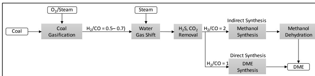
Figure 6 - Schematic Process Flow Diagram of DME Production from Coal (Japan DME Forum, 2011)
