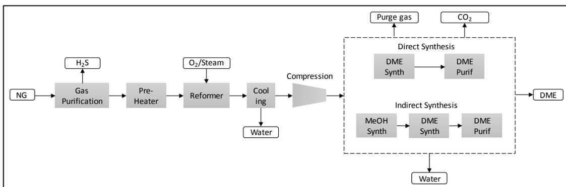
Figure 5 – Schematic Process Flow Diagram of DME Production from Natural Gas (Japan DME Forum, 2011)
