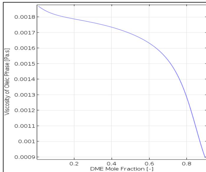
Figure 19 - Viscosity of DME and Hexadecane Mixture using the quarter power law Eqs. (29) and (30)
