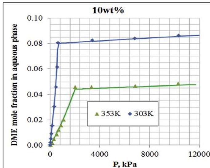
Figure 13 - Solubility of DME in Water at Different Temperatures (Ratnakar *et al.*, 2016a)
