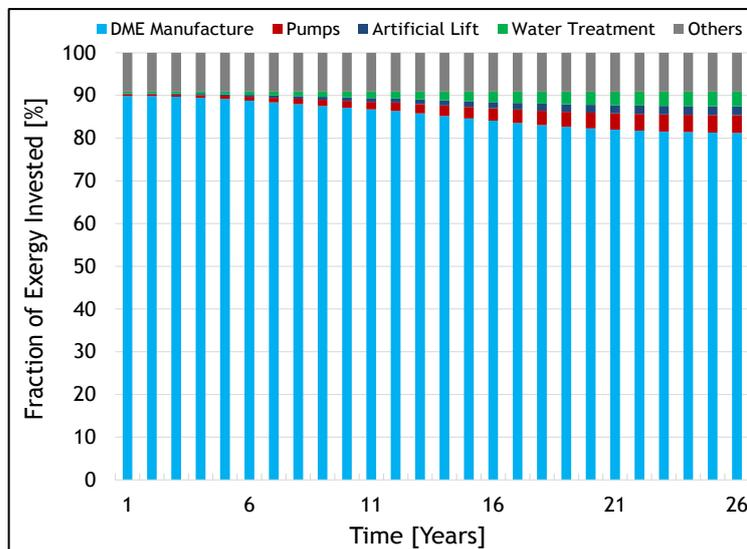
Figure 39 - Fractions of the Invested Exergy in different Components of the Considered System (Cumulative)
