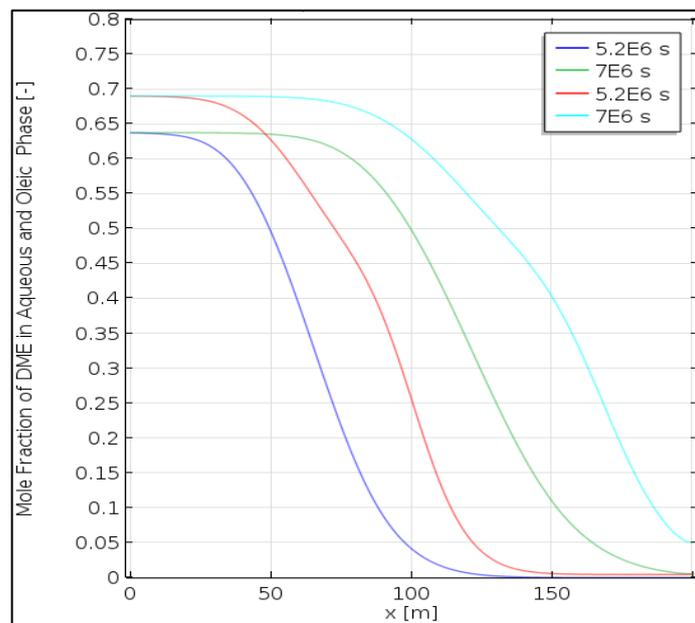
Figure 23 - Mole Fraction of DME in Aqueous Phase (Blue and Green) and Oleic Phase (Red and Cyan)
