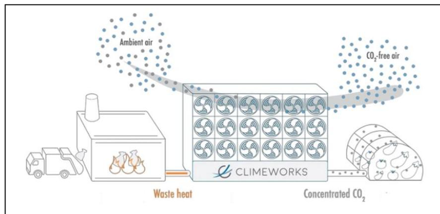
Figure 49 - Climeworks Direct CO<sub>2</sub> Capture Process (Climeworks, 2017)
