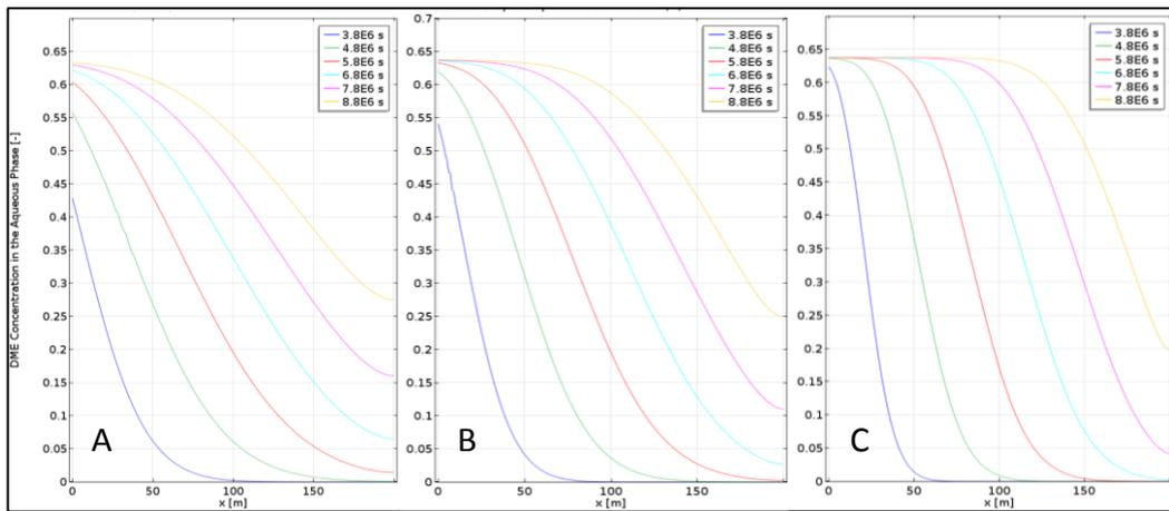
Figure 30 - DME Concentration Profile in the Aqueous Phase [A -  $N_{pe}$  of 5000; A -  $N_{pe}$  of 10000; A -  $N_{pe}$  of 25000]
