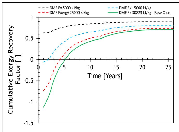
Figure 42 - The Cumulative Exergy Recovery Factor as a function of Time (Sensitivity to Exergy of Manufacturing DME)
