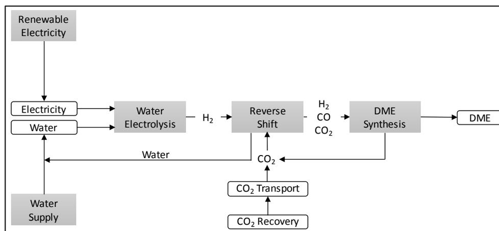
Figure 10 - Flow Diagram of CO<sub>2</sub> Hydrogenation using Renewable Energy (Japan DME Forum, 2011)
