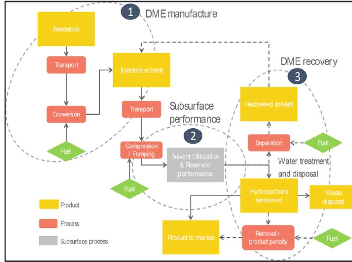
Figure 16 - Schematic Development Lay-out for DEW Process (te Riele *et al.*, 2016)
