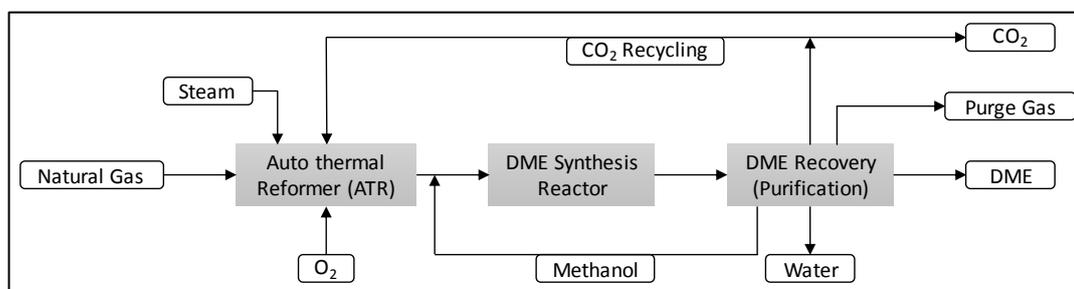
Figure 7 – Flow Diagram of DME Direct Synthesis Process (Japan DME Forum, 2011)
