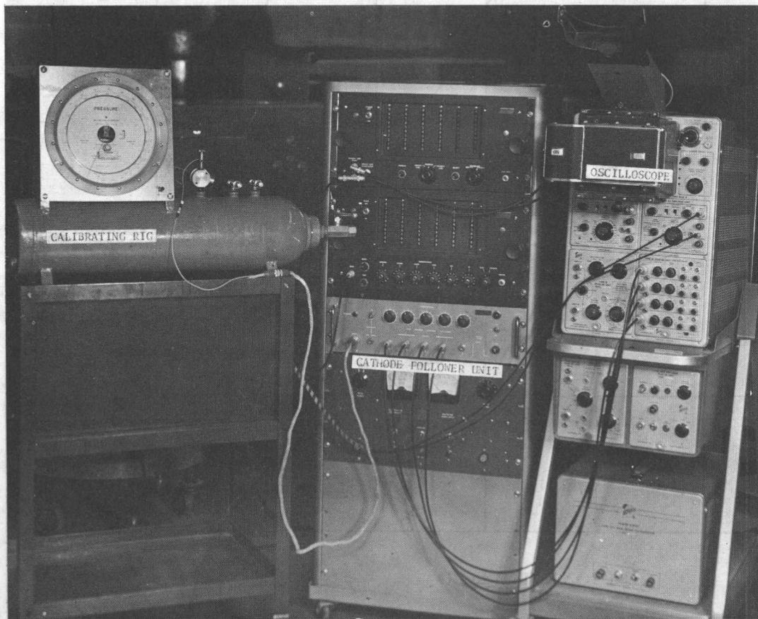
FIG. 67 CALIBRATING RIG FOR PZT PRESSURE TRANSDUCER
