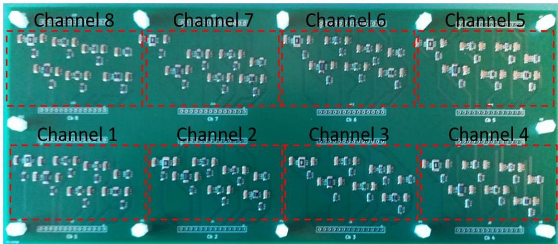
**Figure 39:** The eight channel testing circuit
