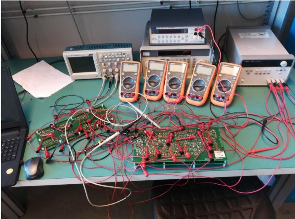
**Figure 40:** Measurements and testing setup of the eight channel neurostimulator (without enclosure).
