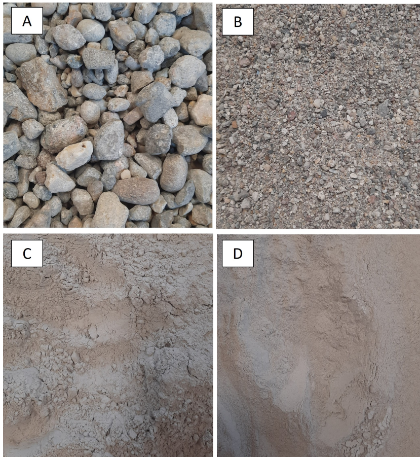
Figure 2.16: Samples of A) Freegravel (4-32 mm), B) Freesand (0.125-4 mm), C) Freefiller (65 - 125 \mu\text{m} ) and D) Freement (0 - 65 \mu\text{m} ) products of the SC system
