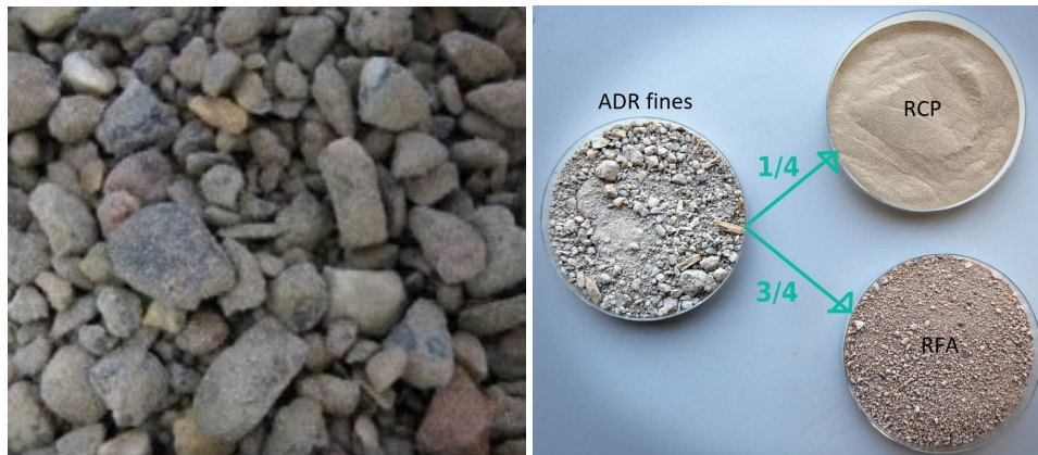
Figure 2.11: Left: ADR coarse (Lotfi and Rem, 2018), Right: HAS input (ADR fines) and output products (RCP and RFA) (TU Delta, 2017)
