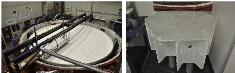
Figure 5: Milled alumina-silica fibre ceramic mould (left) for the casting of the Giant Magellan Telescope mirror blanks and segment of glass produced in such a mould (right)
