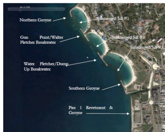
Figure 1.4: Lay-out of the project site, including naming of the structures [Smith Warner International Ltd., 2018].
