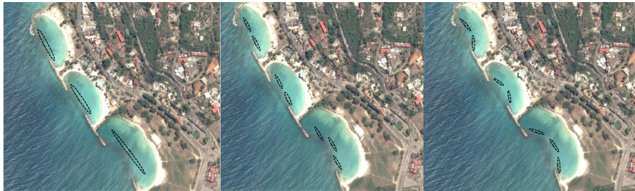
Figure 6.24: Three different submerged breakwater lay-outs [Google 2018]. Left: lay-out 1. Center: lay-out 2. Right: lay-out 3.
