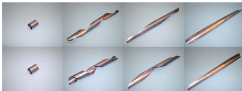
Figure 1.1: Neutrally stable shell[5]
