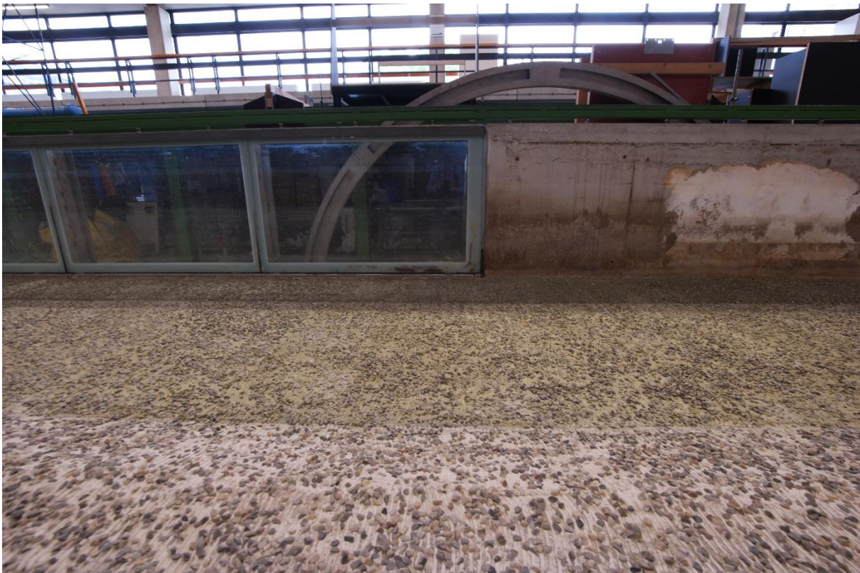
Figure 77; The side wall at the main channel side is concrete for the largest part and a part glass
