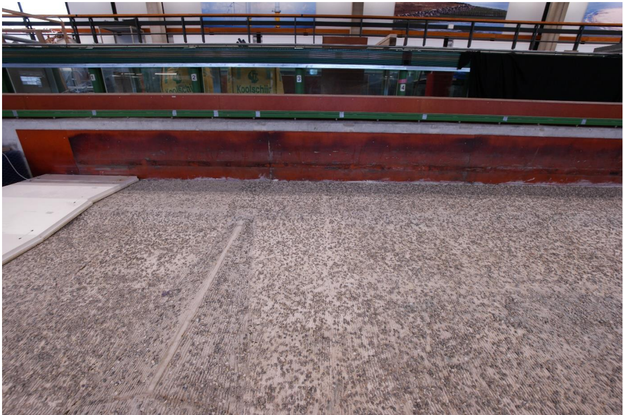
Figure 78; the side wall at the floodplain side are wooden planks
