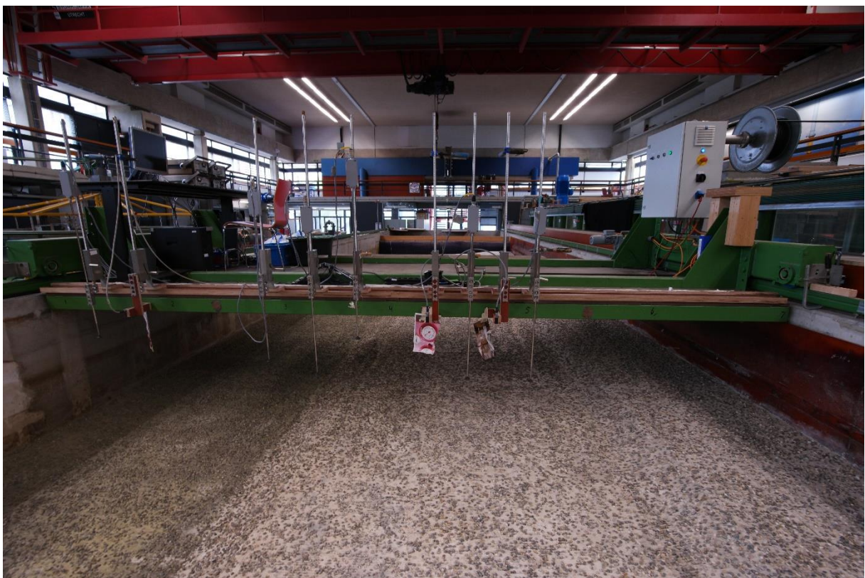
Figure 79; the measurements carriage, with 6 EMS installed and 3 laser altimeters installed
