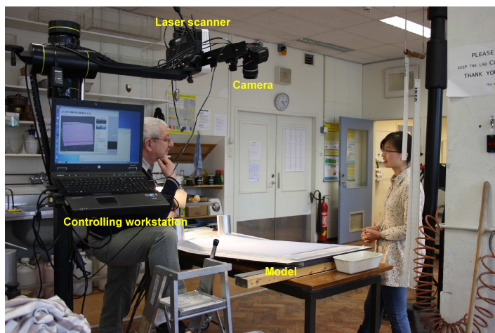
Figure 3.1: Laboratory set-up of the analogue experiments in the ISES tectonic laboratory at the Vrije Universiteit Amsterdam. A computer controlled systems is installed over the sand-silicon model. This system combines a workstation computer for monitoring the experimental process, a laser scanner for collecting the bathymetric data, and a digital camera for taking top-view pictures during the experiments.
