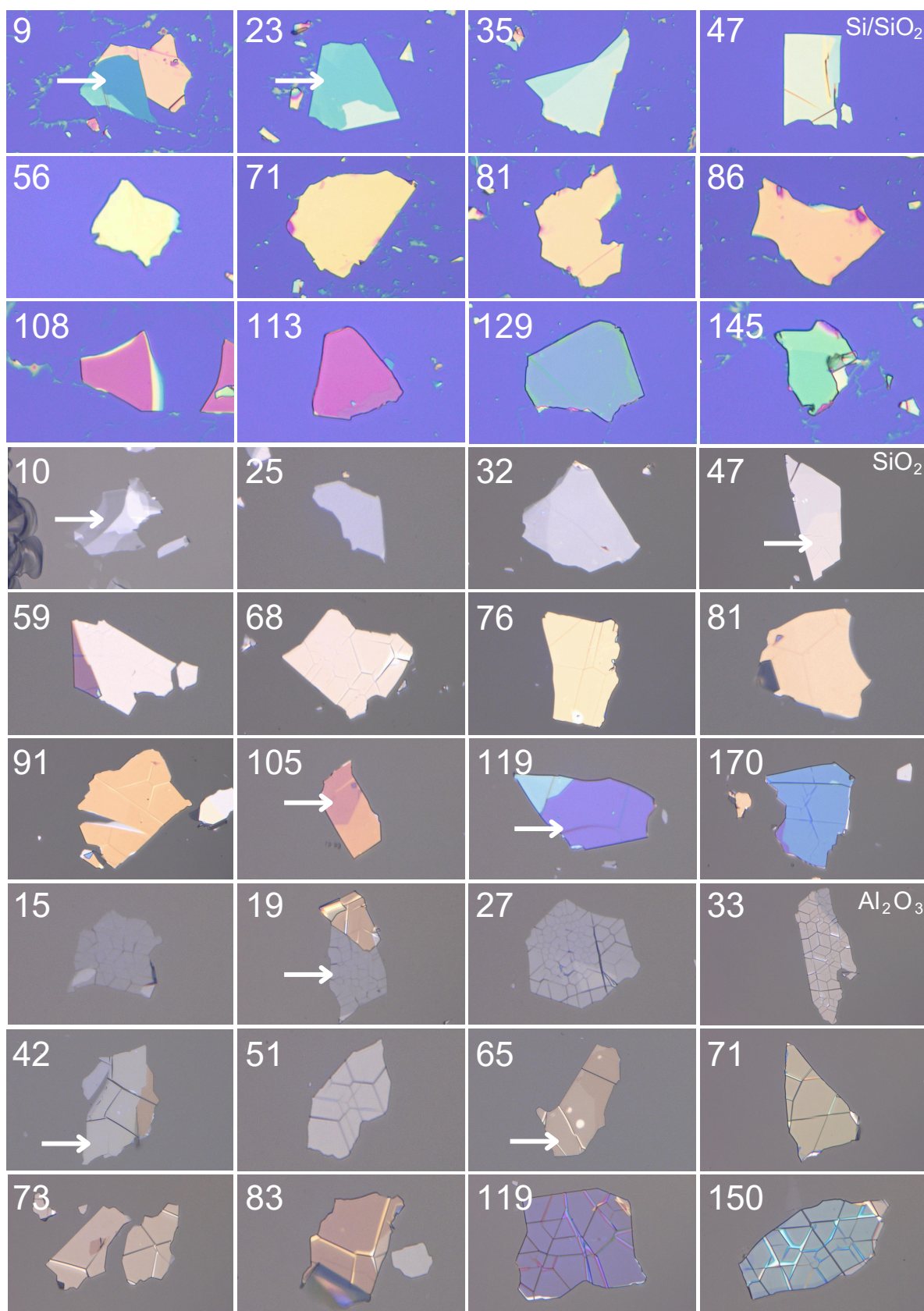
Figure 5.3: Thickness- and substrate-dependent colour of h-BN on Si/SiO 2 , quartz (SiO 2 ), and sapphire (Al 2 O 3 ). The figure shows a mix of pre- and post-annealed flakes, explaining the variations in wrinkle density. The flake thickness (in nanometers) is indicated in the top left corner, with arrows pointing to the relevant regions when multiple thicknesses are present. Images were captured using the Keyence VHX-6000 microscope with combined coaxial lighting and a brightness setting of 50. Flake thickness was determined with AFM.
