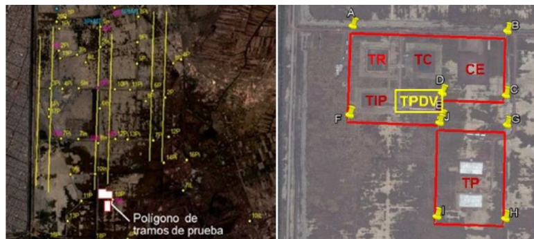
Figure 6.1: On the left side the location of the trial embankments at the NAICM site [2]. On the right side the positions of the trial embankments with respect to one another. In yellow the position of the TPDV embankment (Terraplén de prueba con Precarga y Drenes Verticales) is highlighted, this is the embankment with sandpiles and PVDs on each side.
