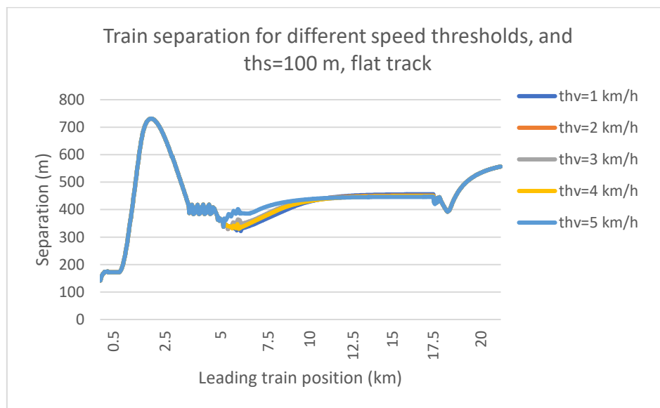
Figure B.2 Train separation for different speed thresholds, flat track
