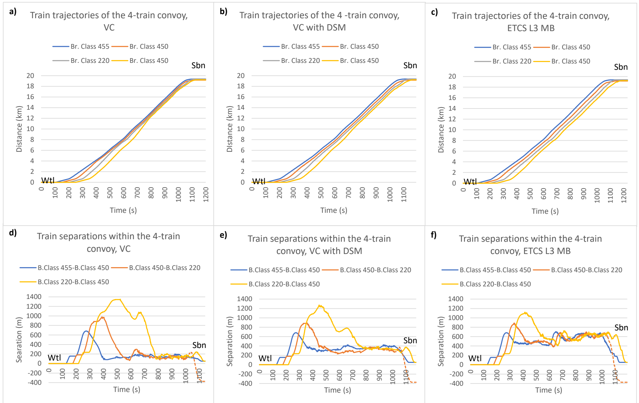
Figure 6.21 Train trajectories (a,b,c) and train separations between trains (d,e,f) for VC , VC considering a DSM and ETCS L3 MB, WTL-SBN with 1 stop at SBN
