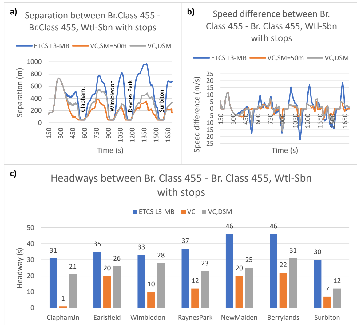
Figure 6.4 Train separation (a), speed difference (b) and headways (c) for Suburban-Suburban, WTL-SBN with stops
