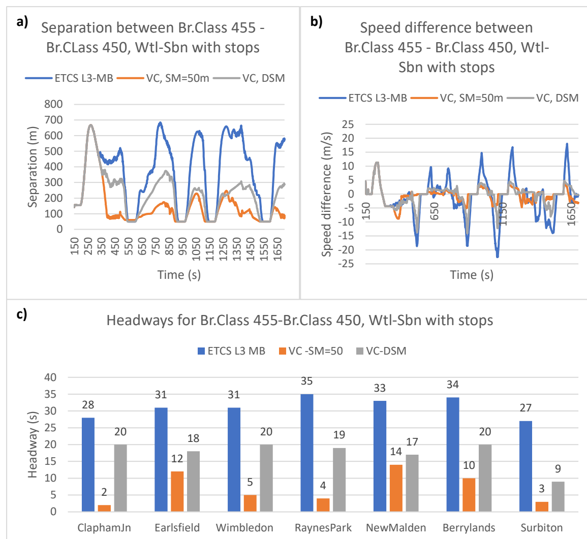
Figure 6.12 Train separation (a), speed difference (b) and headways (c) for Suburban-Regional, WTL-SBN with stops
