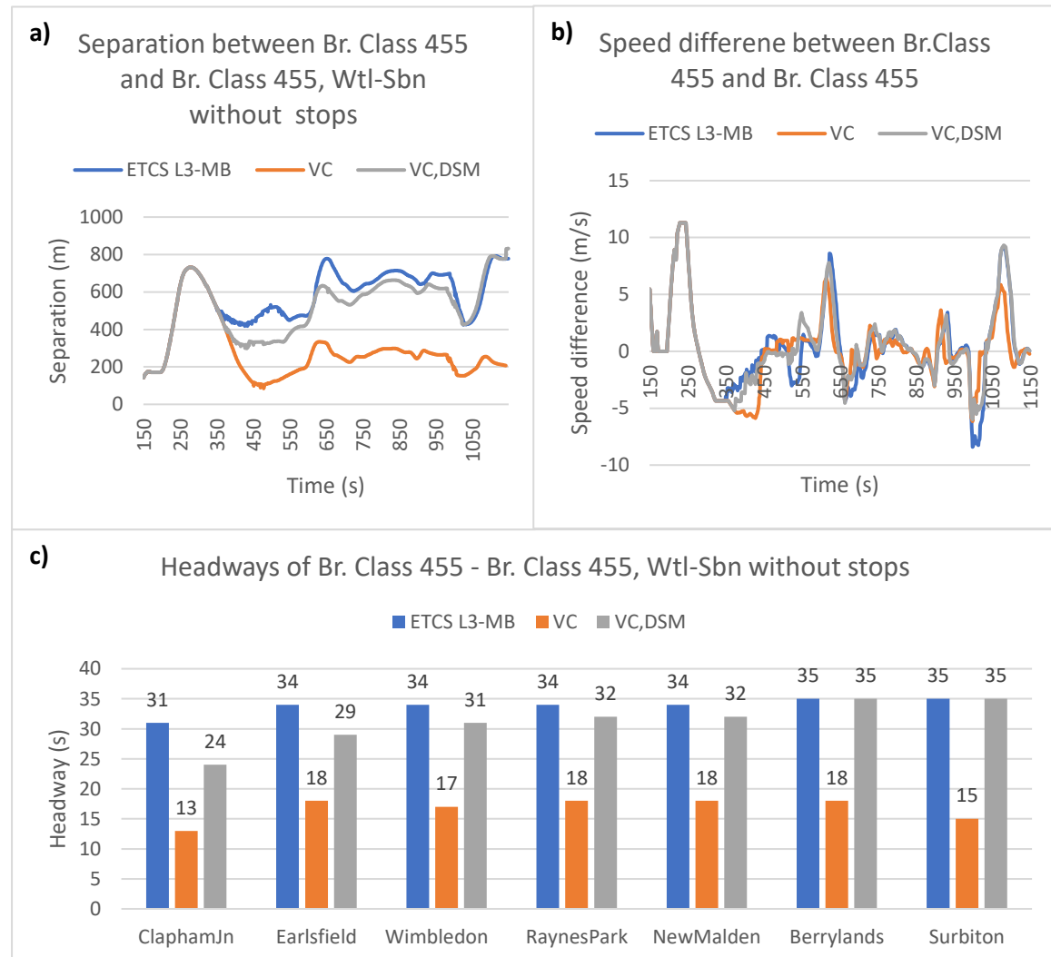
Figure 6.3 Train separation (a), speed difference (b) and headways (c) for Suburban-Suburban, WTL-SBN without stops
