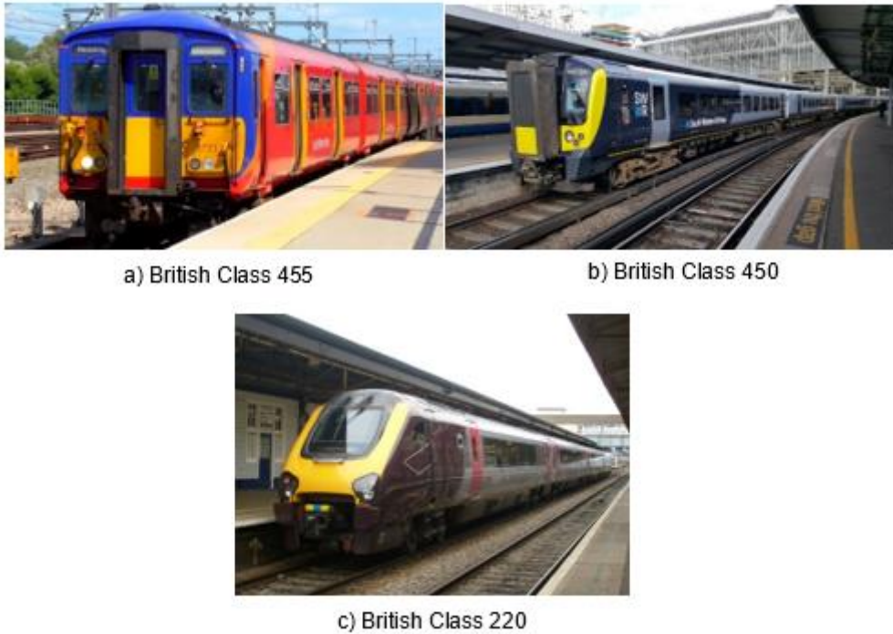
Figure 6.1 a) British Class 455 (commuter train), b) British Class 450 (regional train), c) British class 220 (intercity train)
