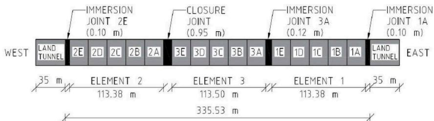
Figure 1. Long section through Kil tunnel showing the element locations, segment numbering and location of joints (from Rijkswaterstaat 1974).
